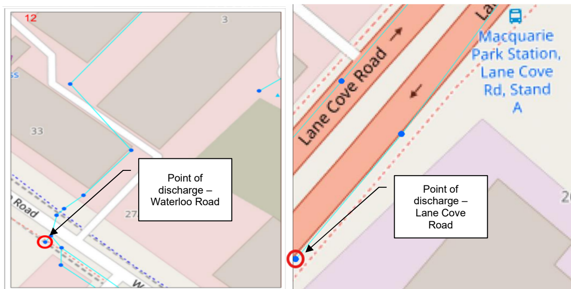
Figure 6-1: Existing connection pit location (Source: City of Ryde Council drawings, Before You Dig Australia)
