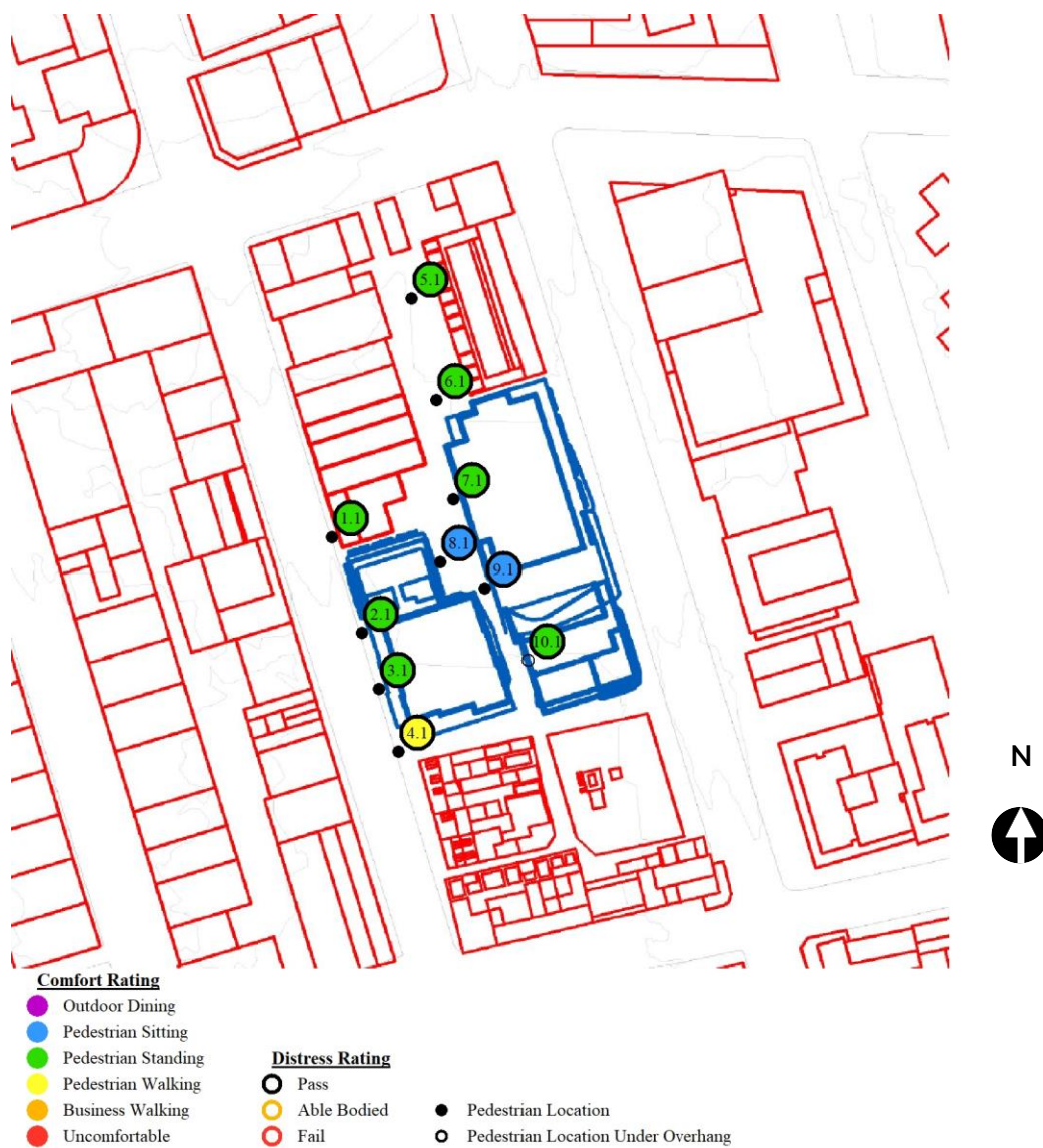
Figure 5: Pedestrian wind speed measurement locations with comfort/safety ratings – Surrounds – Configuration 2.
