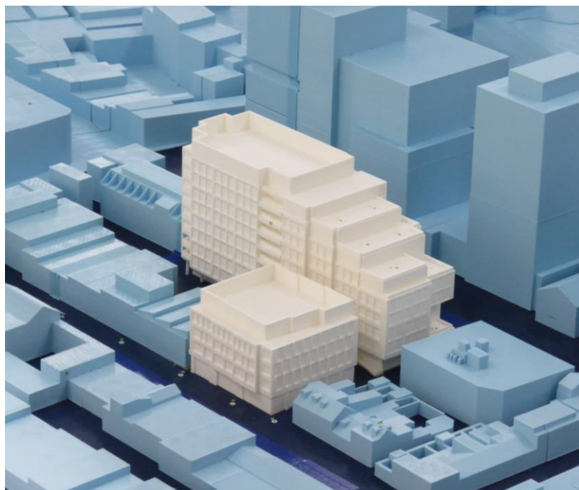
Figure 1b: Photographs of Wind Tunnel Test Model, close-up – Configuration 1 (top) and Configuration 2 (bottom).
