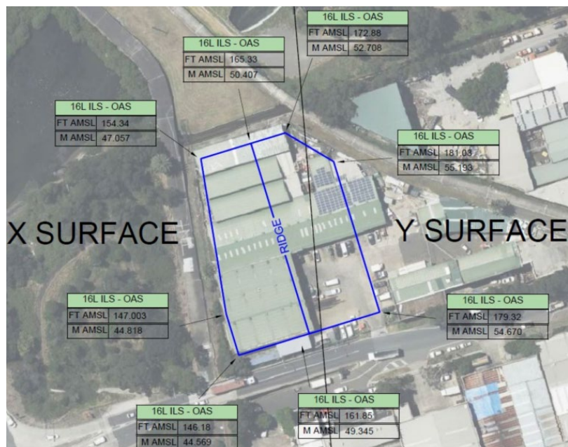
Figure 9: PANS-OPS - X and Y surfaces (16L Approach)
