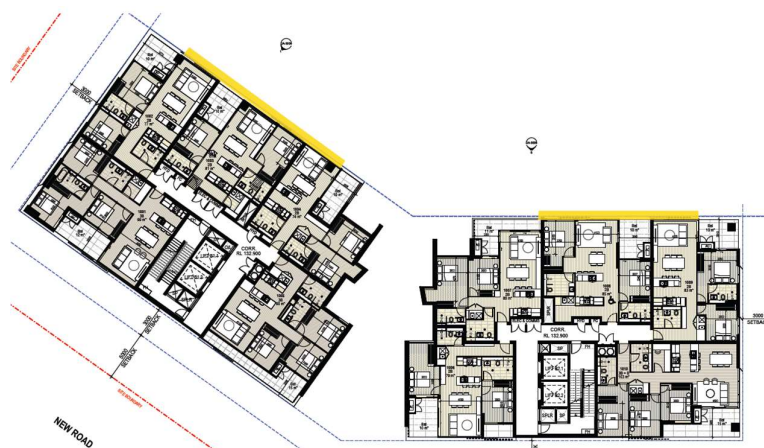
Figure 5: Plan of sunhood locations on towers B1 and B2 which protrude beyond the approved envelope by approximately 150mm (Source: Group GSA)
