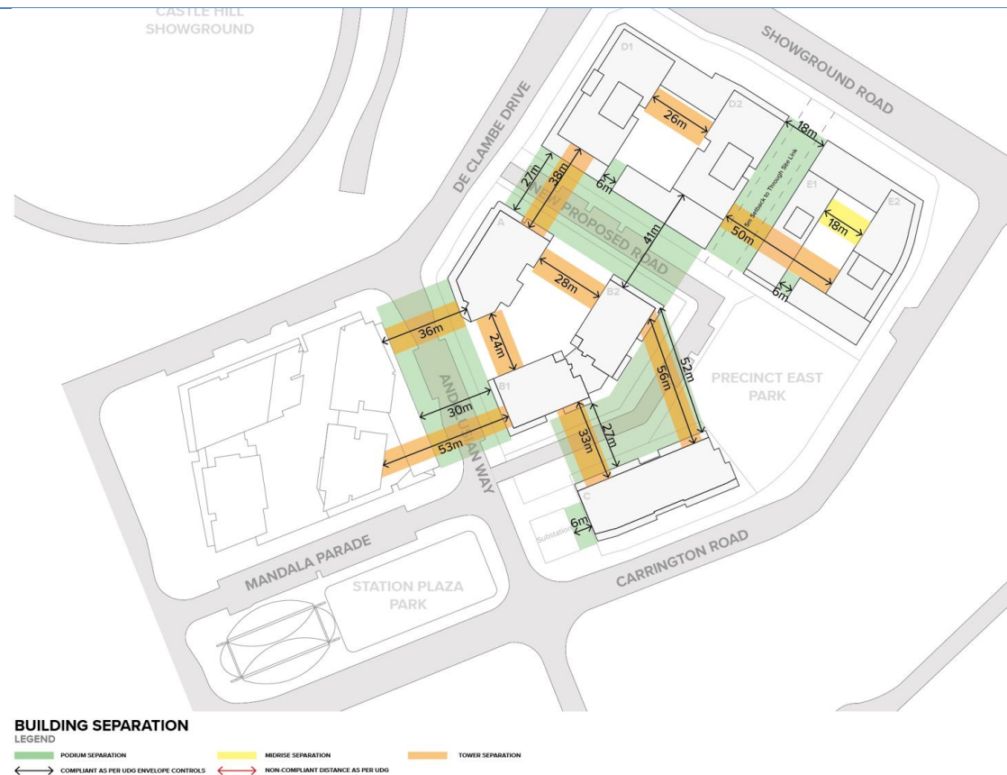
Figure 34: Proposed Building Separation (Source: Turner Studio)
