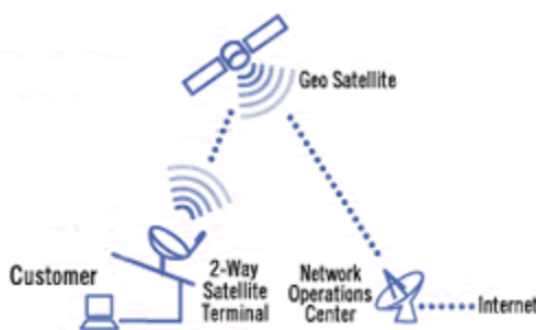
Figure 2: Two way connection to the Internet via Satellite [23]
