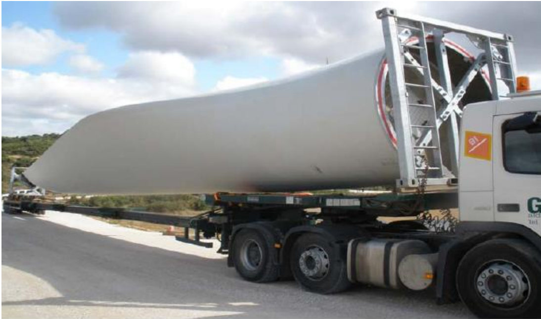
Figure 4.3: Typical Over Dimensional Load (Blade Section)
