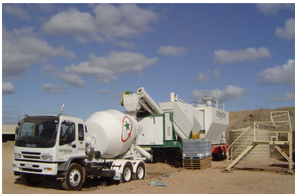
Figure 4.6 Portable batching plant - Modular silo batching plant
