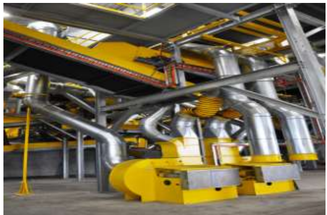
Figure 9: Blowers used to remove any light waste
