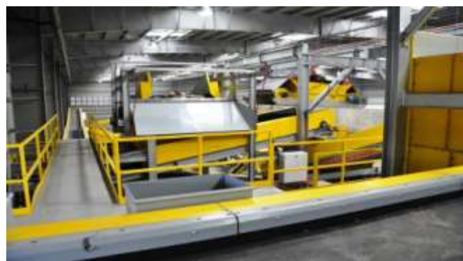
Figure 5: Long object separator
