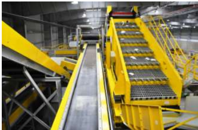
Figure 7: Waste screen which separates material into over 65cm and under 65cm
