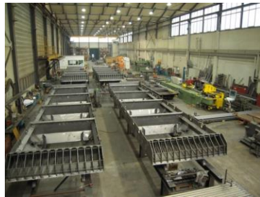
Fig. 5.5 c – Zones of a grate being manufactured in the KRB workshop (KRB)
