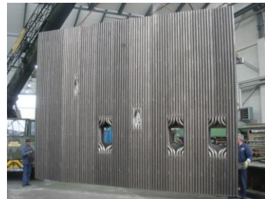
Fig. 5.5 d – Manufactured and ready-to-install membrane wall with burner openings (KRB)
