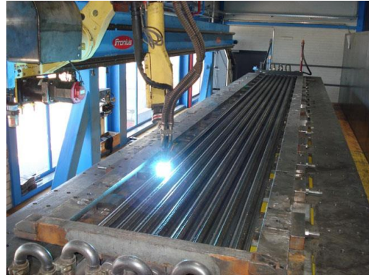
Fig.5.5 a - Robot for welding Inconel cladding onto membrane walls (KRB)
