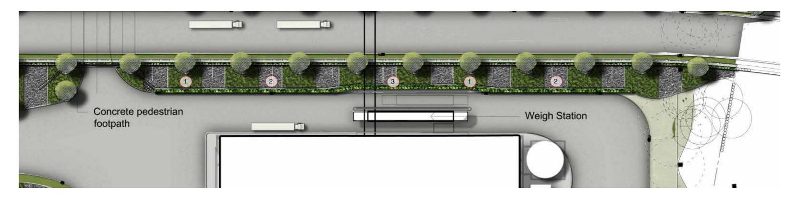
The weigh-bridge area is located against the level change up to street level. Using a ballast and planting stabilized slope eliminates the cost of a retaining structure, and creates a bold repeating pattern of rock and ground cover planted bands across the slope. This softens the outlook for staff and truck drivers who occupy this area 24/7.
