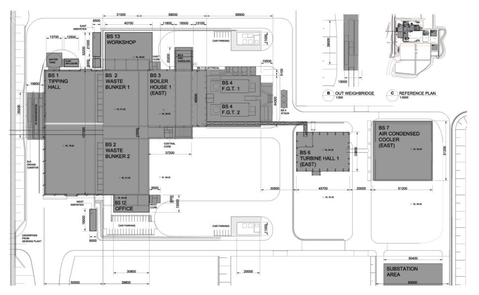
FIGURE 5 – DIMENSIONS OF PROJECT COMPONENTS (SOURCE: KTA)
