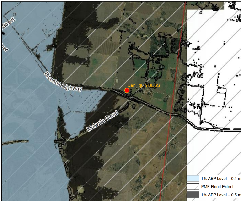
Figure 8-1 Riverine Flood Planning Level extent (Figure 32; WMAwater 2014)
