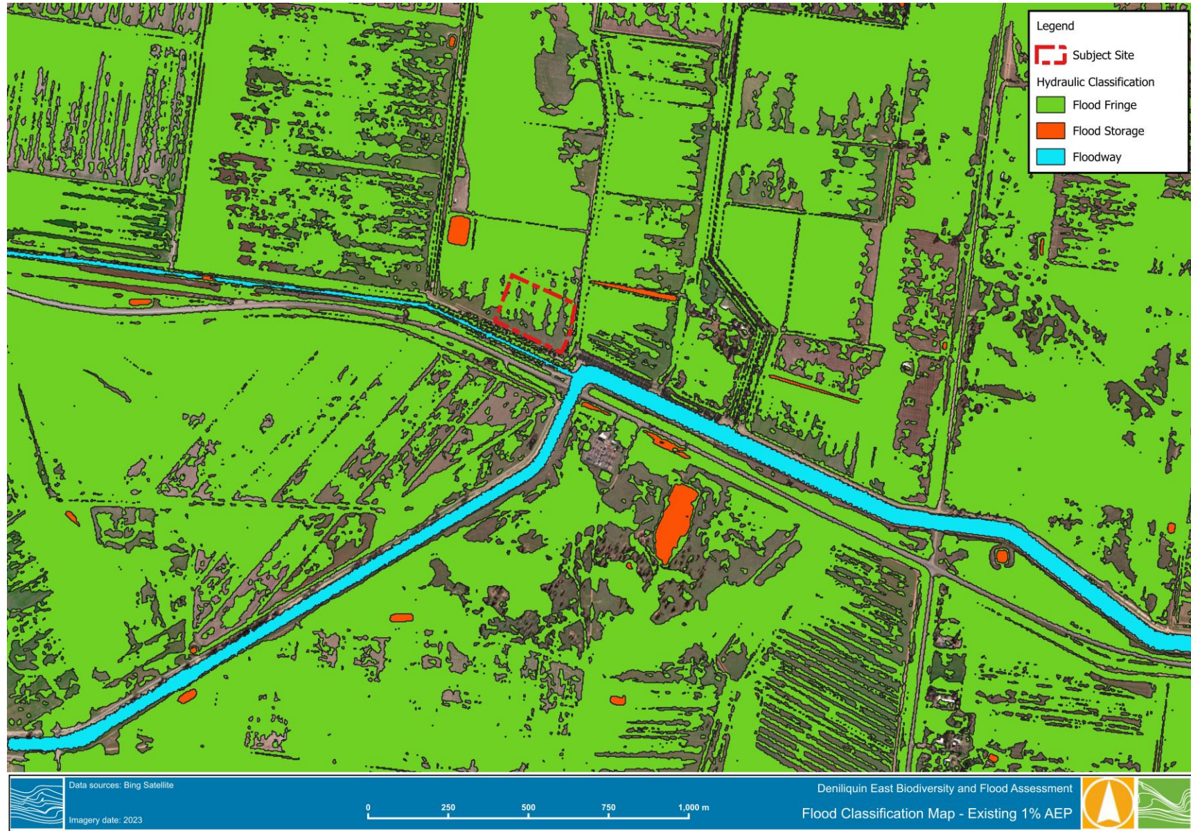
Figure 5-6 Existing Conditions – 1% AEP flood classification
