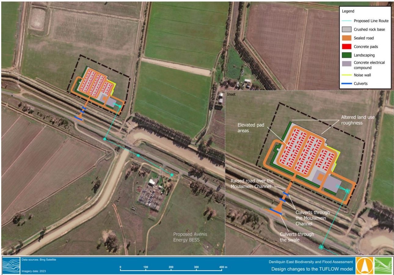
Figure 3-7 Hydraulic model changes for the design scenario
