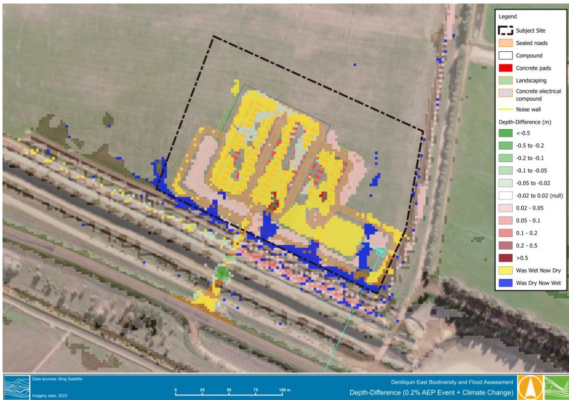
Figure C 5 Design Conditions – 0.5% + climate change AEP depth-difference
