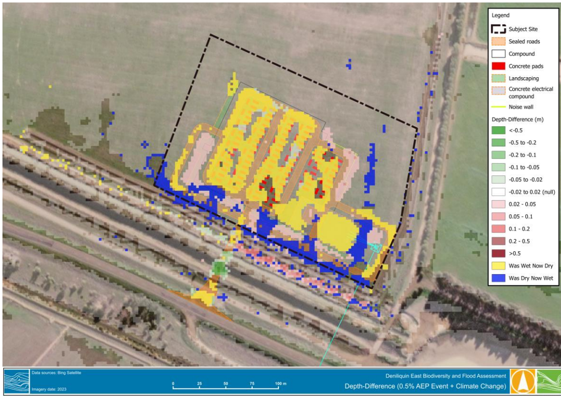
Figure C 5 Design Conditions – 0.5% + climate change AEP depth-difference
