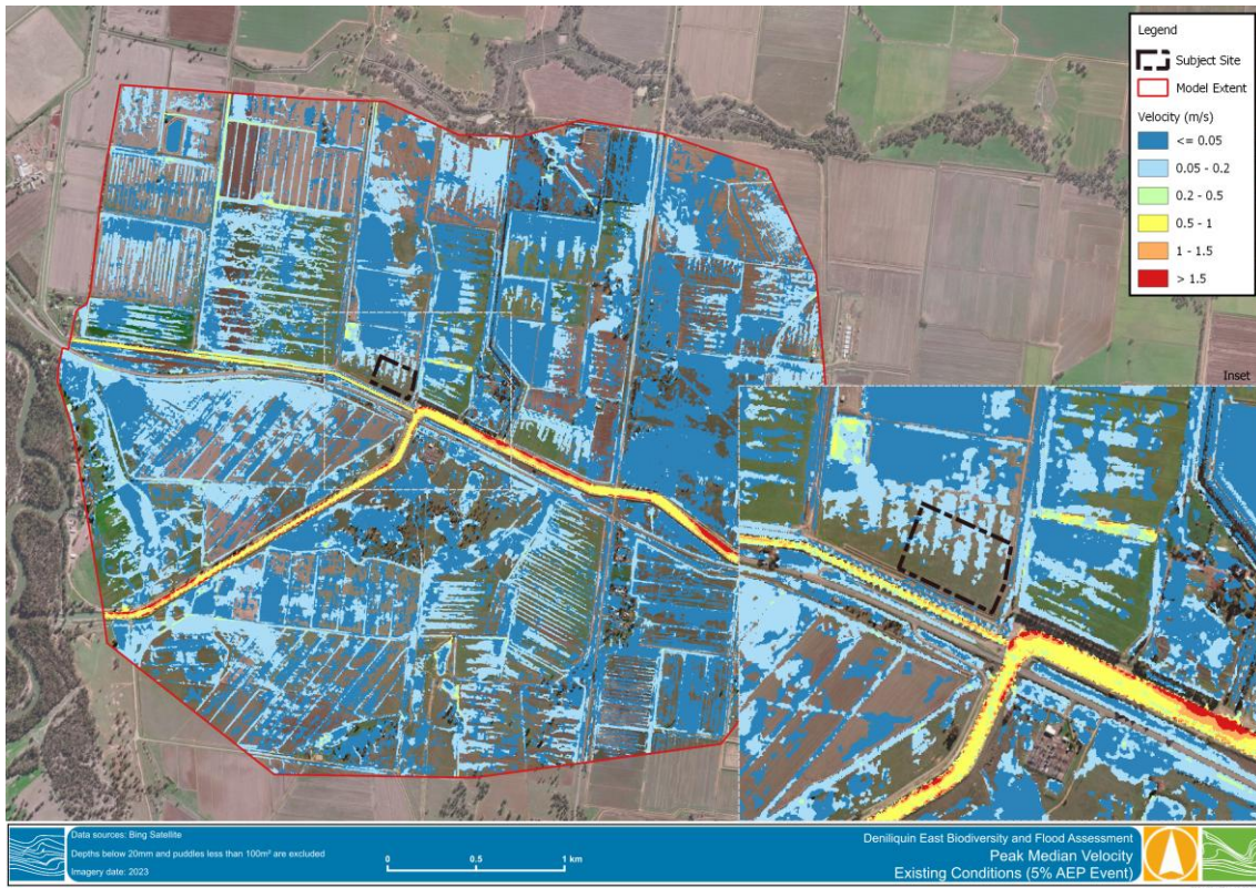
Figure B 5 Existing Conditions – 5% AEP flood velocity
