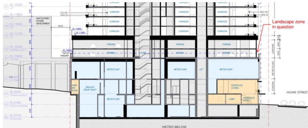
Figure 3: Original SSDA Design – Hume St section
