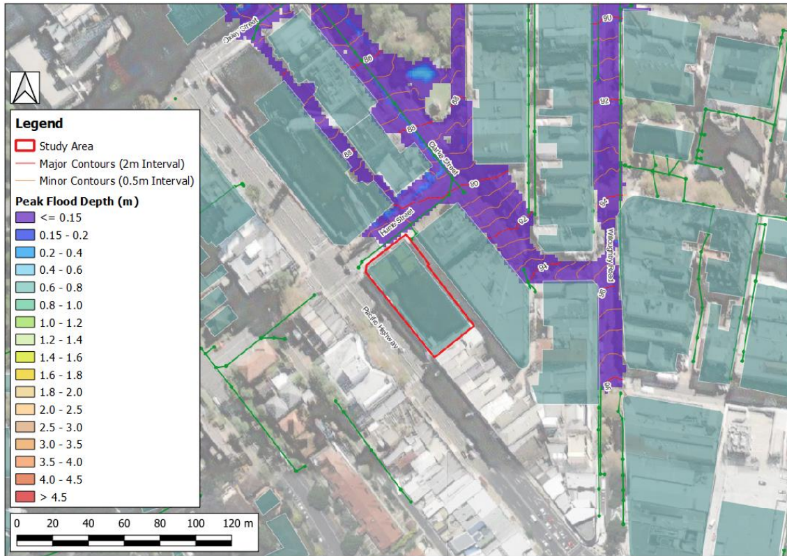
Figure 19 – 1% AEP Event Flood Depth and Level Contours (RCP 8.5 Scenario with 0.9m Increase in Sea Level – Post Development Scenario)
