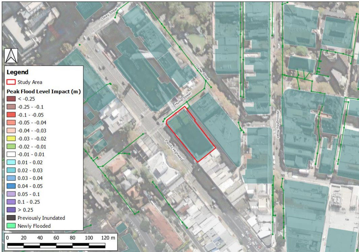
Figure 21 – 1% AEP Event Peak Flood Level Impact (RCP 8.5 Scenario with 0.9m Increase in Sea Level)
