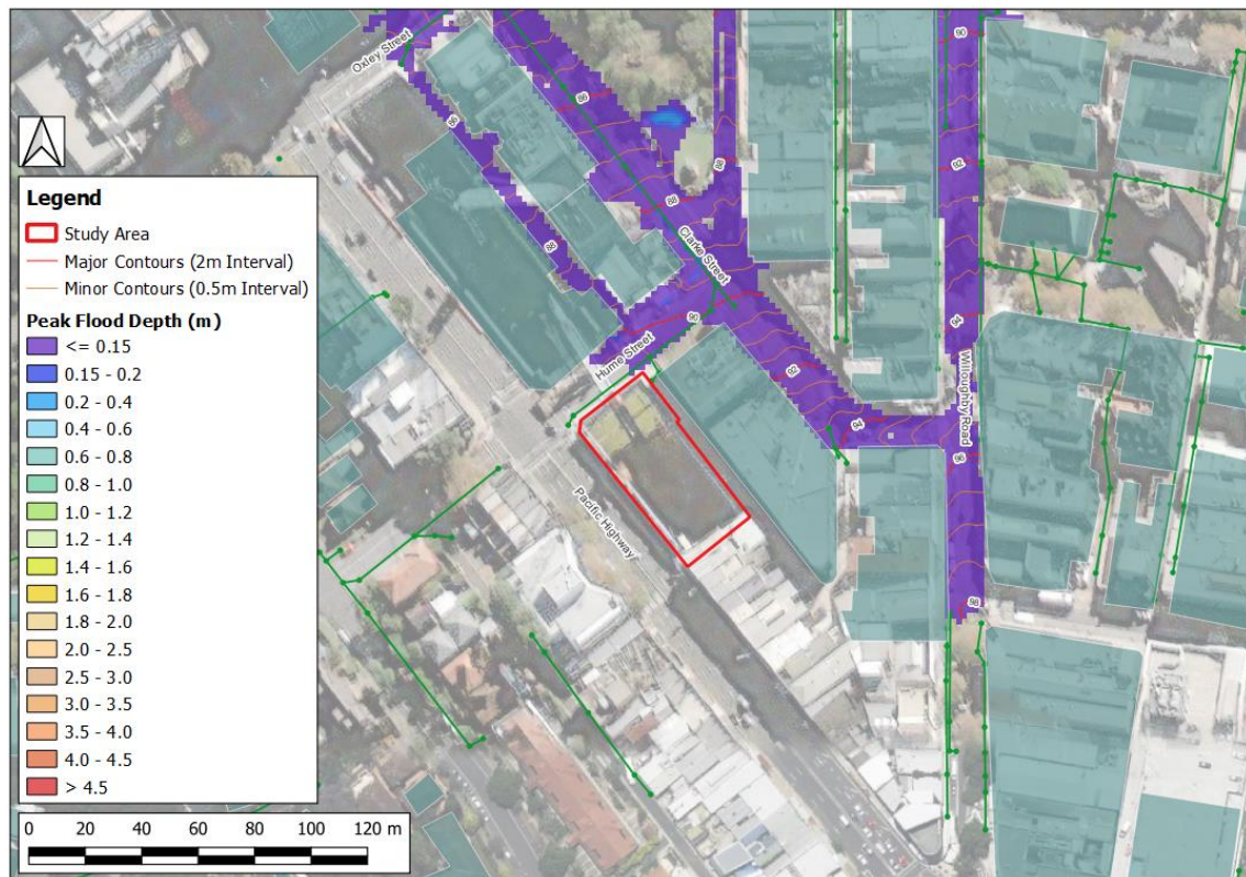
Figure 17 – 1% AEP Event Flood Depth and Level Contours (RCP 8.5 Scenario with 0.9m Increase in Sea Level – Pre-Development Scenario)
