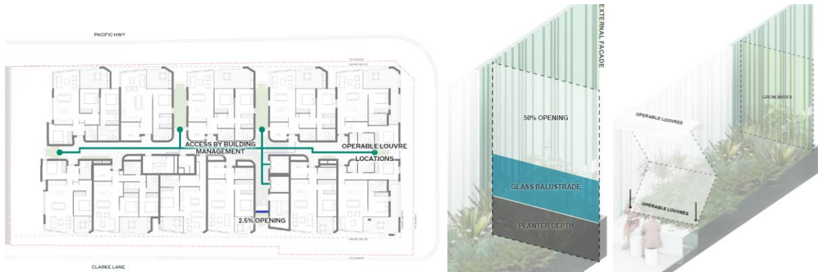
Figure 14: Corridor openings (Levels 7+) – operable louvre locations (L), openable area (M), operable louvres inside of planters (R)
