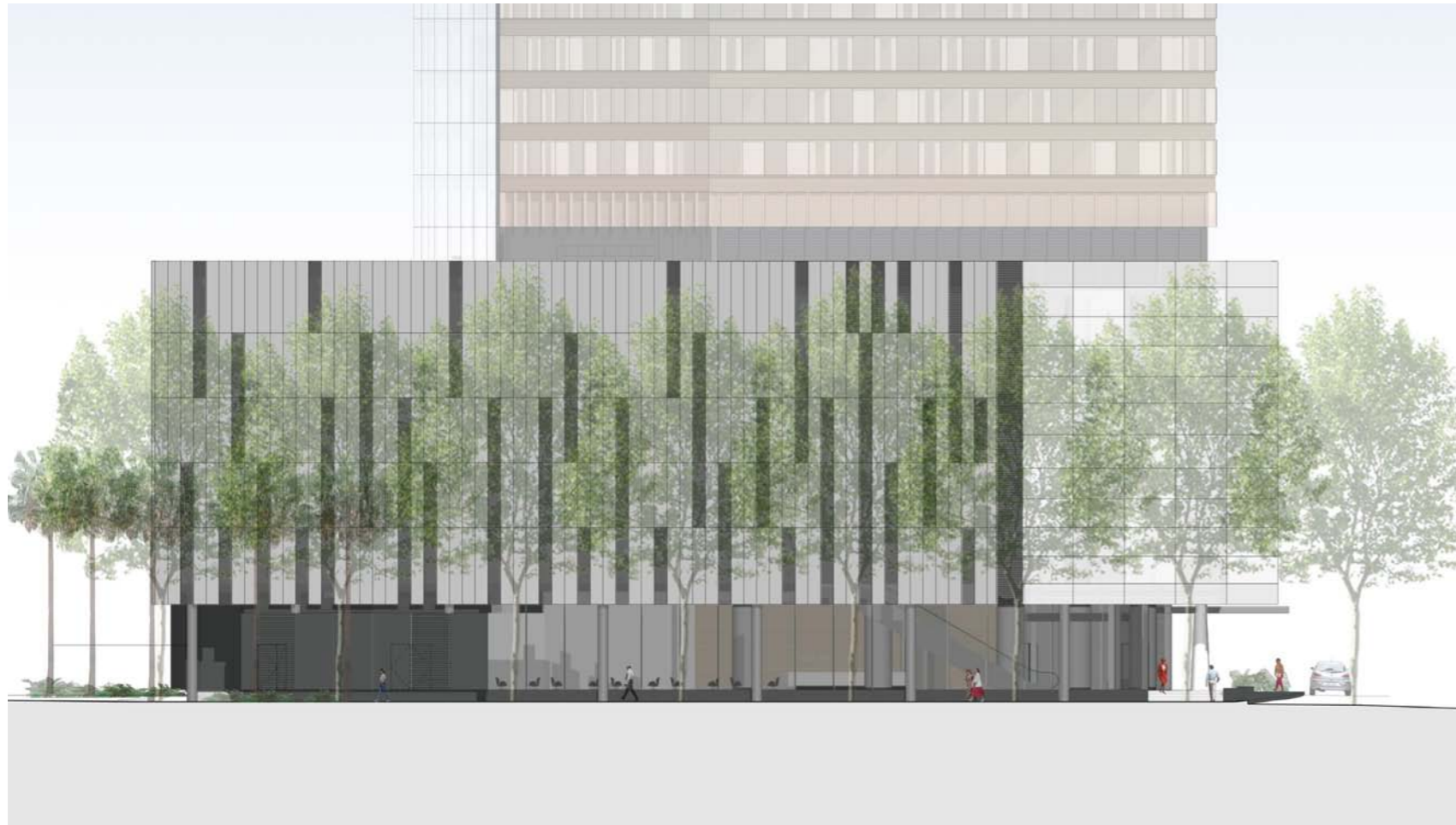
Elevation of northern podium volume. The fenestration pattern allows a wide range of functions to be accommodated behind a single facade system, responding to increased requirements for daylight with a locally increased density of glazing.
