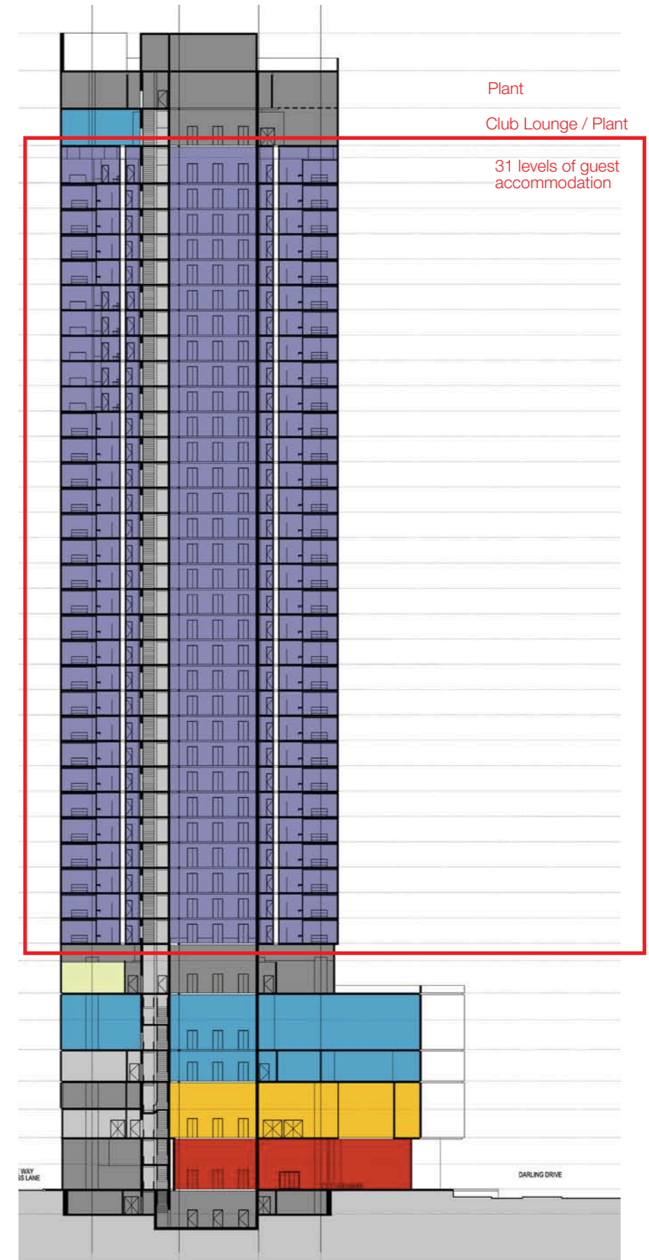
Typical Cross Section showing hotel rooms levels
