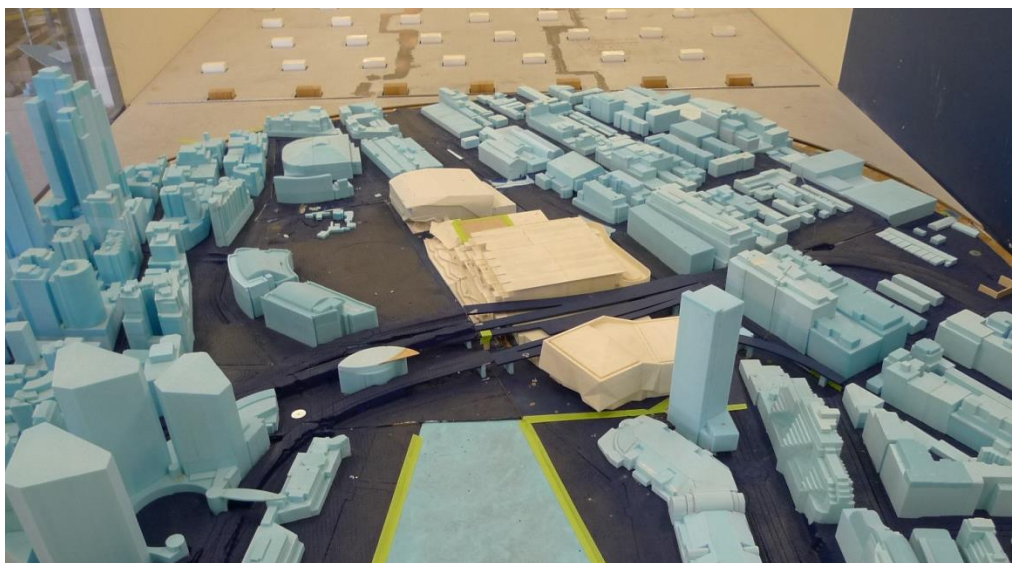
Figure 4: Configuration A in the CPP wind tunnel – View from the North
