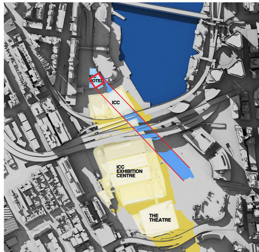
Tower orientation minimises width of shadow at key times
