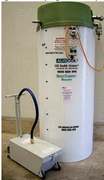
Figure 6 – Oil recycling silo and transport caddy
