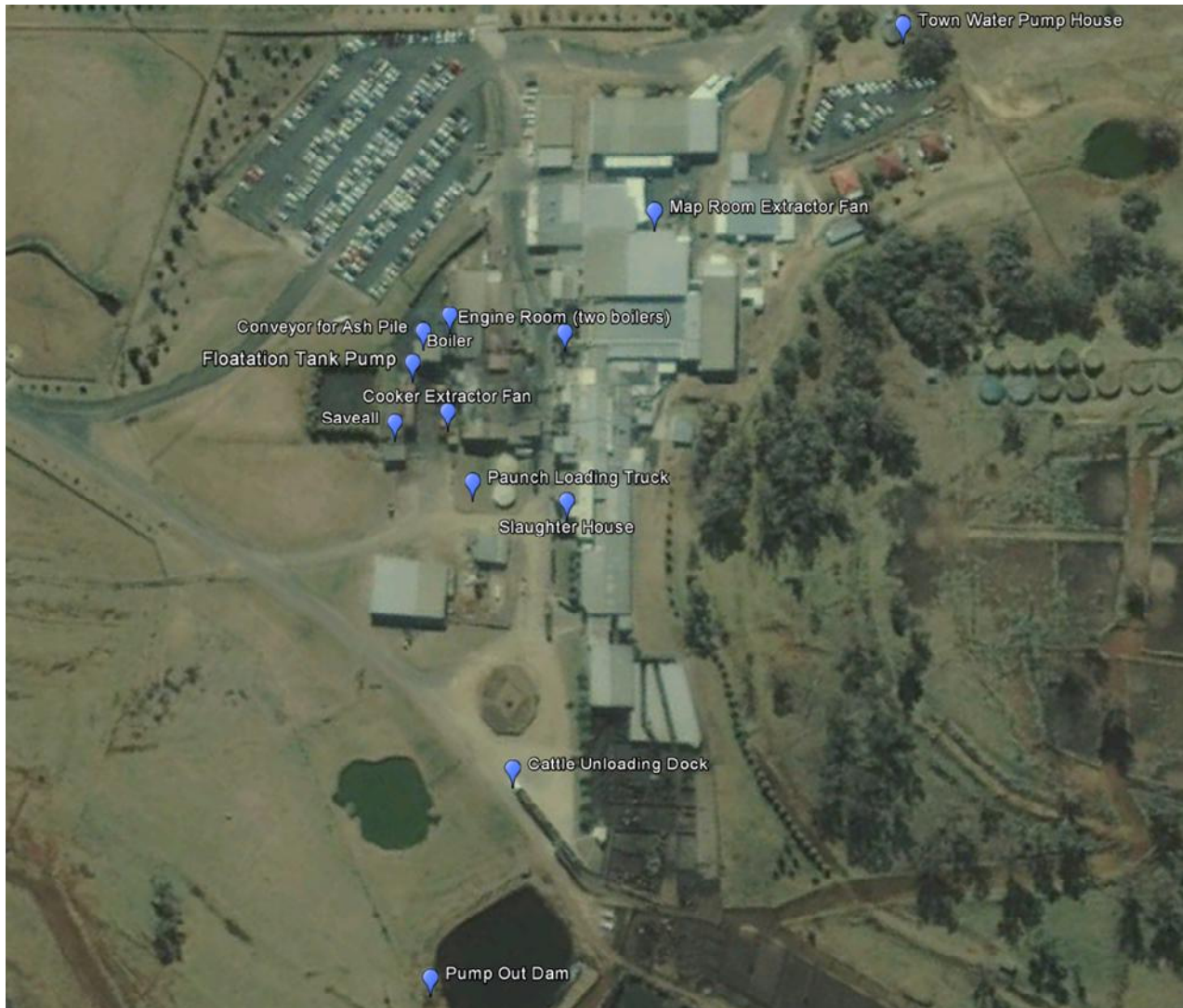
FigureD-1: Existing Noise Source Locations [Google Earth]
