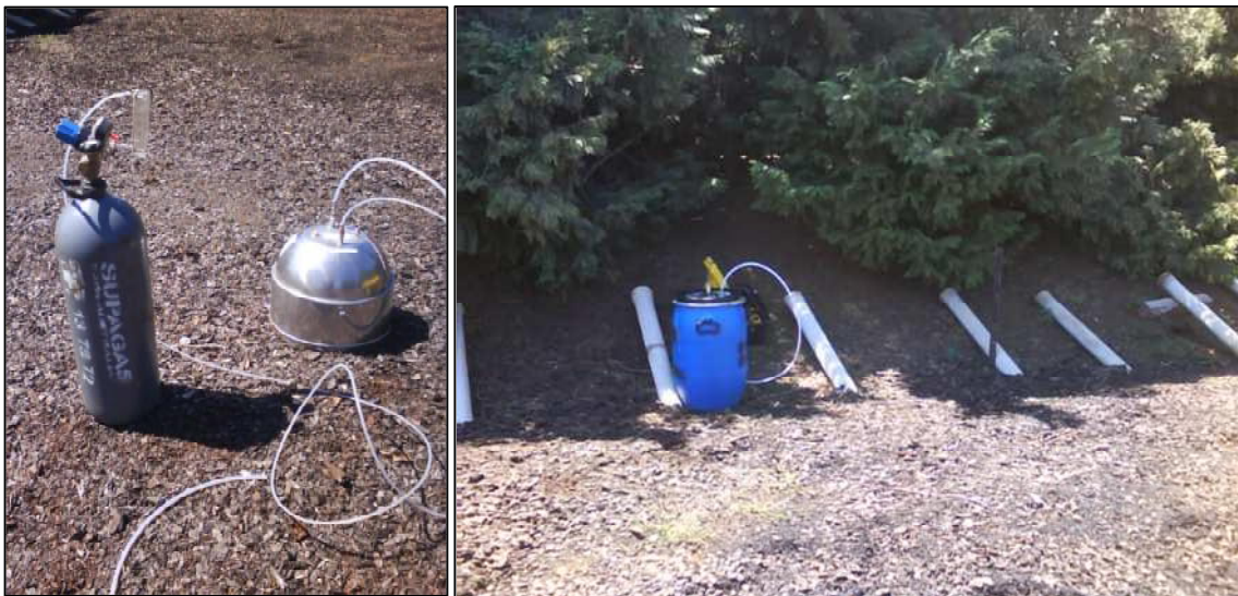
Figure 4-2: Sampling the Bio-filter Surface and Feed Air [Vipac 2013]
