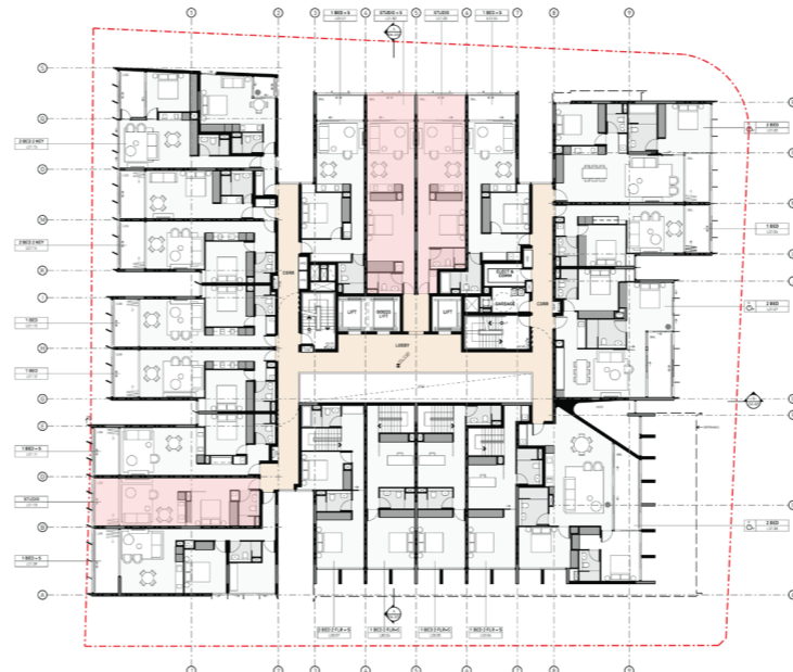
DA104 LEVEL 1 FLOOR PLAN no. of single aspect apartments = 3 no. of south facing apartments = 0
