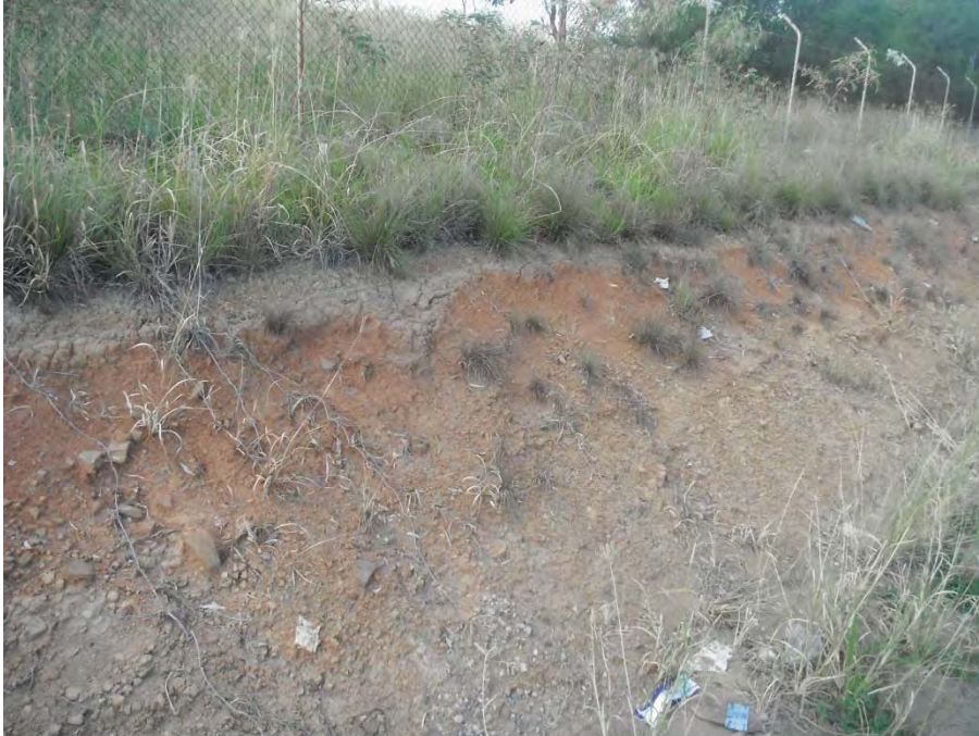
Plate 1: soil profile in road batter, east side of Old Wallgrove Road near Austral Bricks. Clay soil grading to weathered shale
