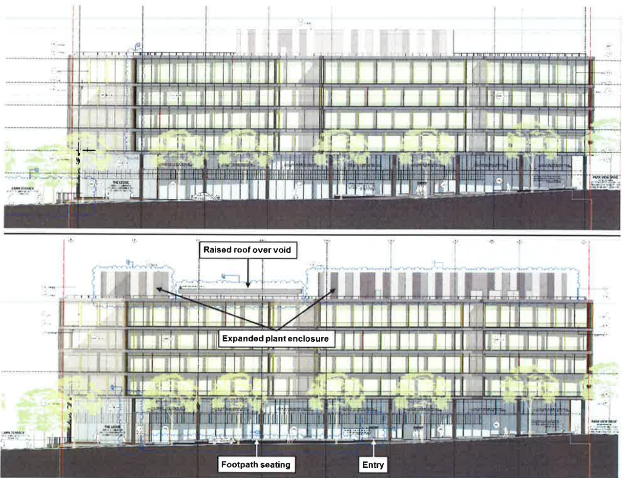
Figure 5: Approved (top) and proposed (bottom) northern elevation (Source: SSD 6076 MOD 1 and applicant's EIS)
