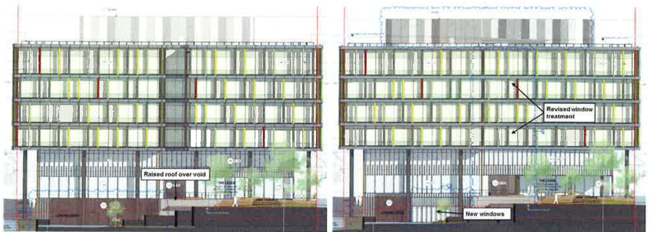
Figure 4: Approved (left) and proposed (right) eastern elevation (Source: SSD 6076 MOD 1 and applicant's EIS)
