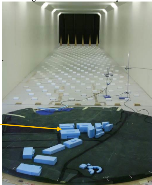
Figure 6: Photograph of wind tunnel model for 5 Murray Rose Avenue
