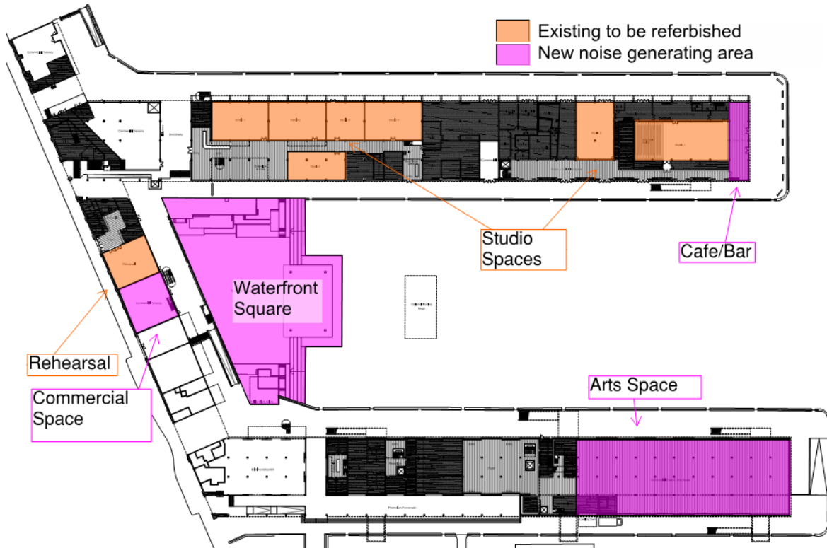
Figure 10 - Existing and new noise generating areas - ground
