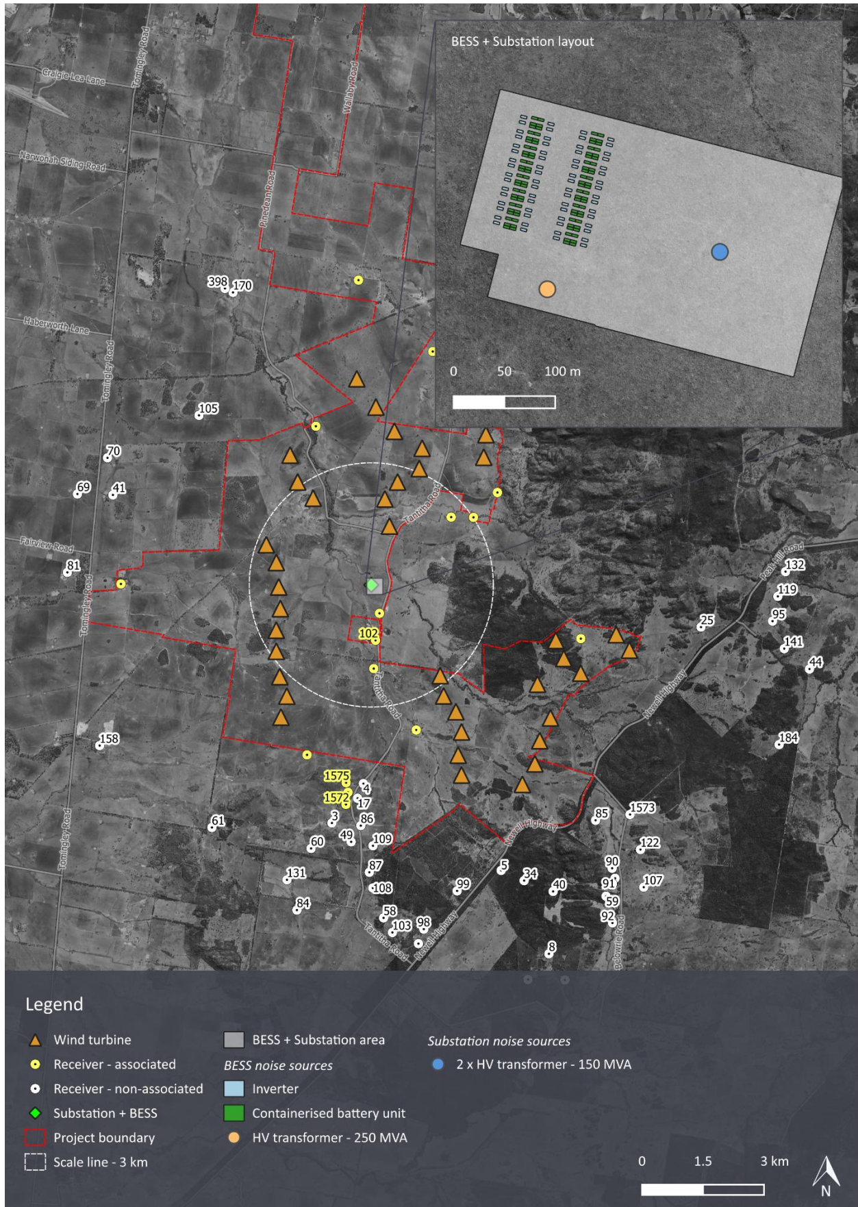
Figure 4: Ancillary infrastructure noise source overview
