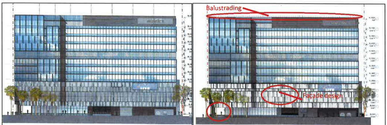
Figure 5: Comparison of approved (left) and proposed (right) external façade changes. Source: applicant's EIS).
