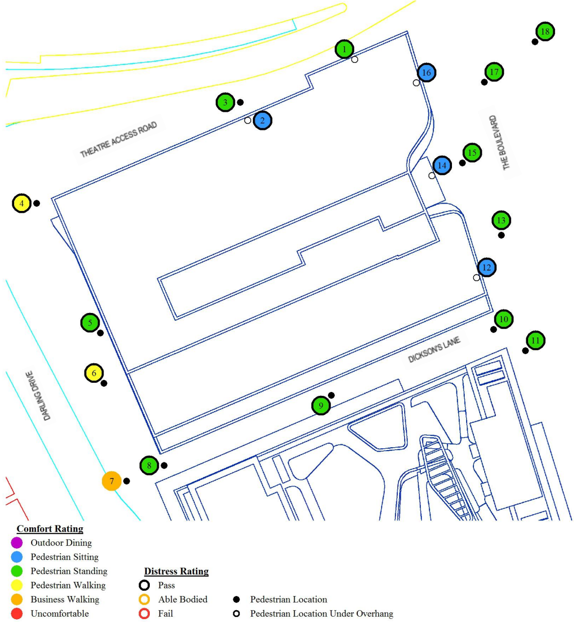
Figure 7: Pedestrian wind speed measurement locations with comfort/distress ratings – Ground Level
