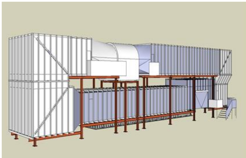
Figure 3: Schematic of the closed circuit wind tunnel
