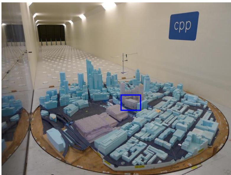
Figure 5: Proposed SICEEP PCP model in the wind tunnel viewed from the northwest
