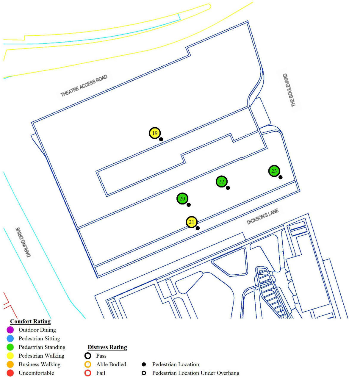
Figure 8: Pedestrian wind speed measurement locations with comfort/distress ratings – Roof
