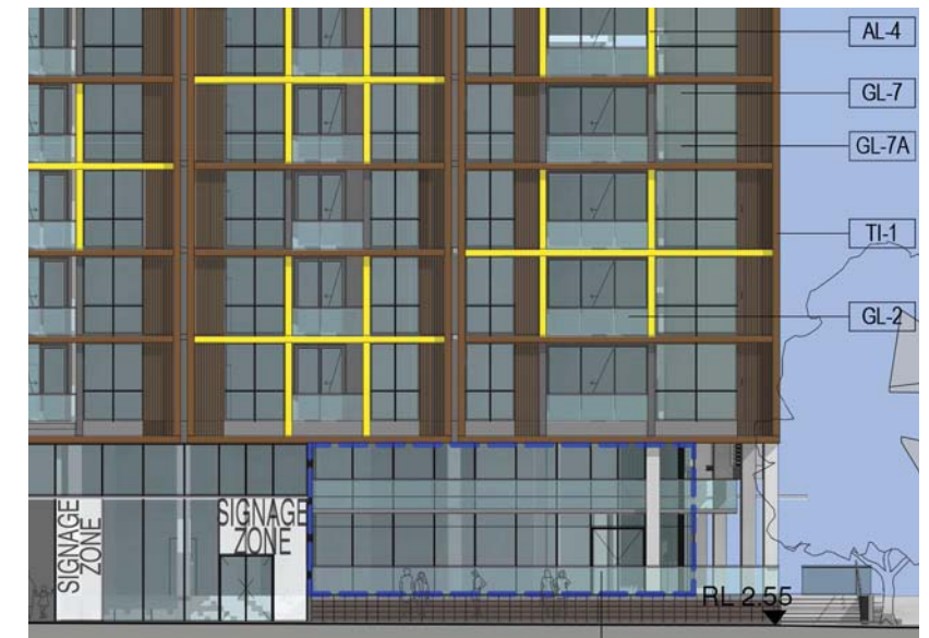
SW2 lobby signage zones - east elevation
