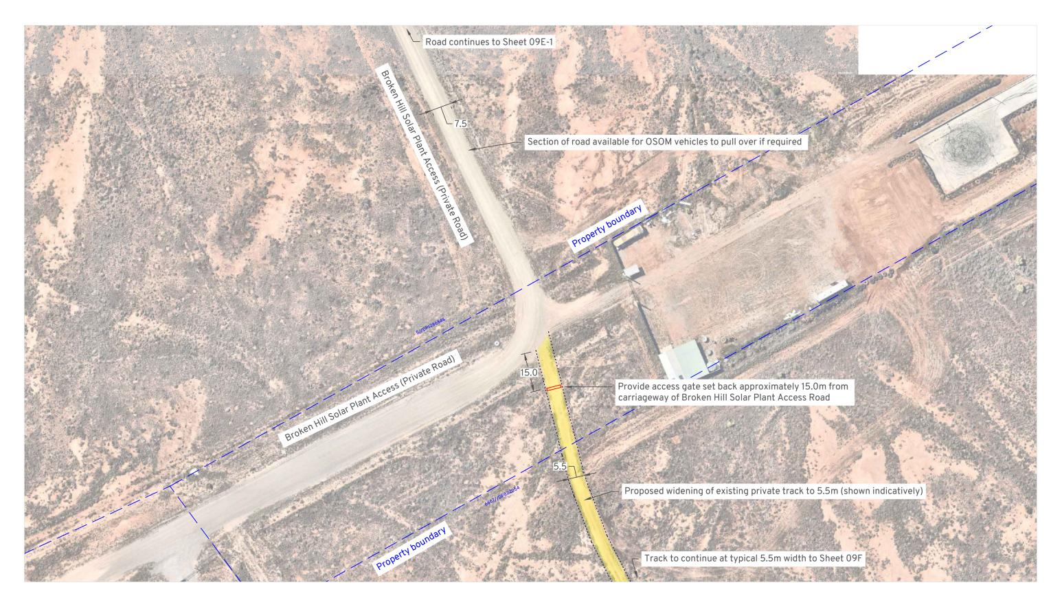
Access gate to remain closed at all times except when required for Project traffic. Property boundaries shown indicatively based on mapping data.
