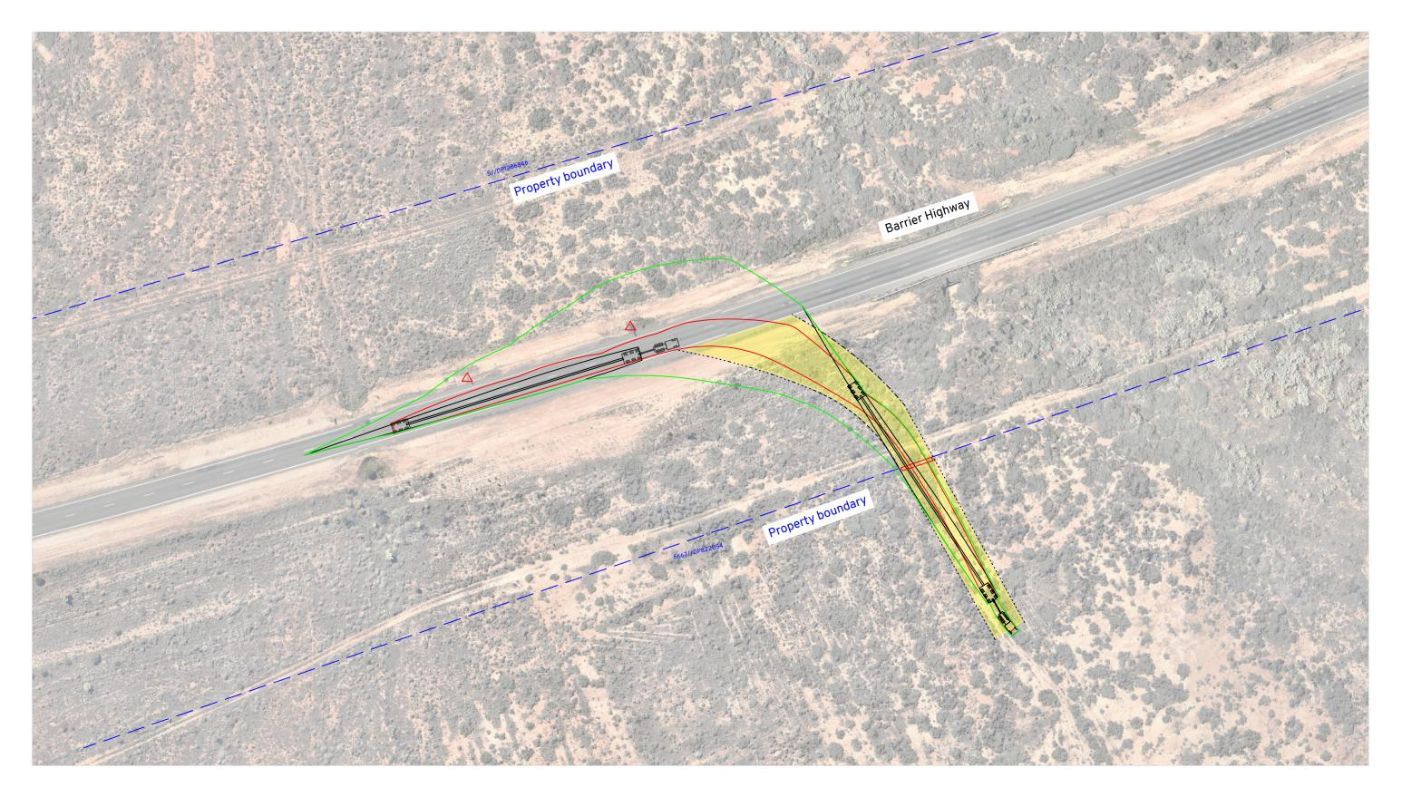
Red = Vehicle wheel path. Green = Turbine blade swing path. Refer to Ares report for detailed OSOM vehicle specifications.
