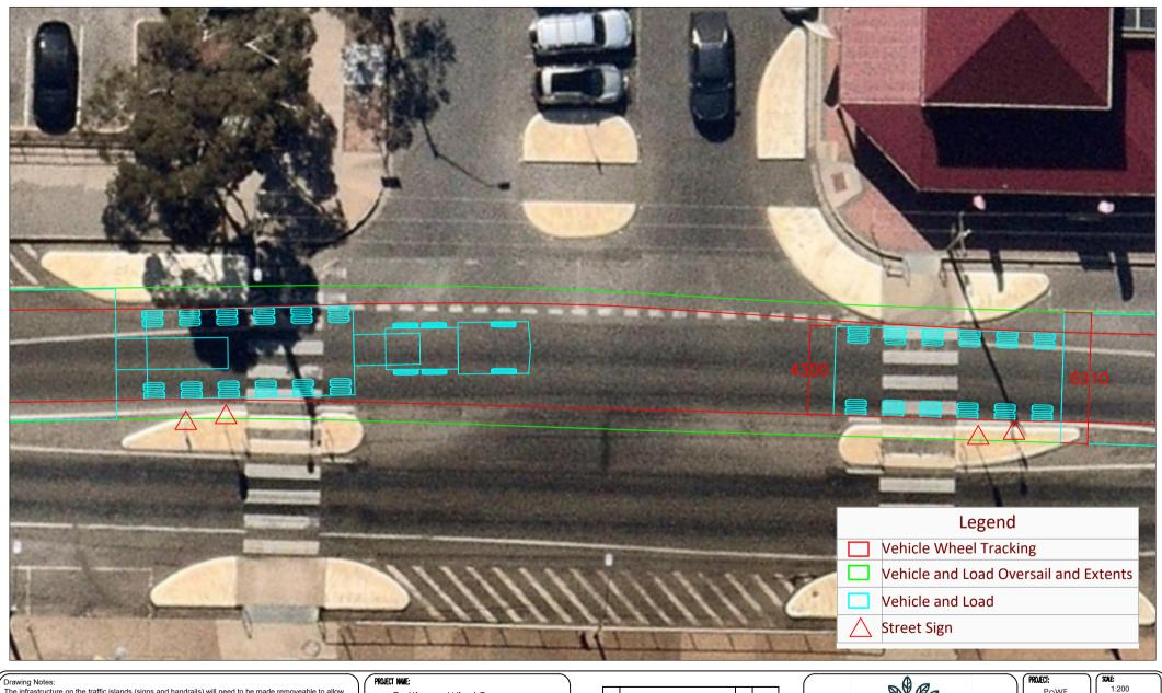
The infrastructure on the traffic islands (signs and handrails) will need to be made removeable to allow the tower to pass.
