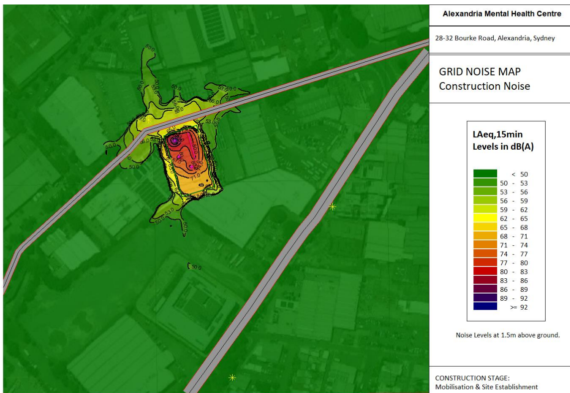
Figure 9-1 Grid noise map showing predicted construction noise – Mobilisation Stage
