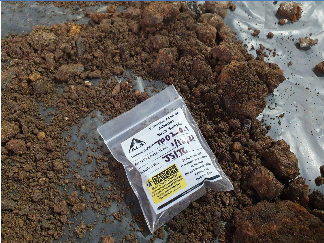
Plate 7 – Representative image of Soil material observed during SCA (EP Risk 2021): Gravelly clayey sand, low to medium plasticity, fine to medium grained, angular to sub-angular gravels, dark brown with red mottling, slightly moist, soft, loose consistency.
