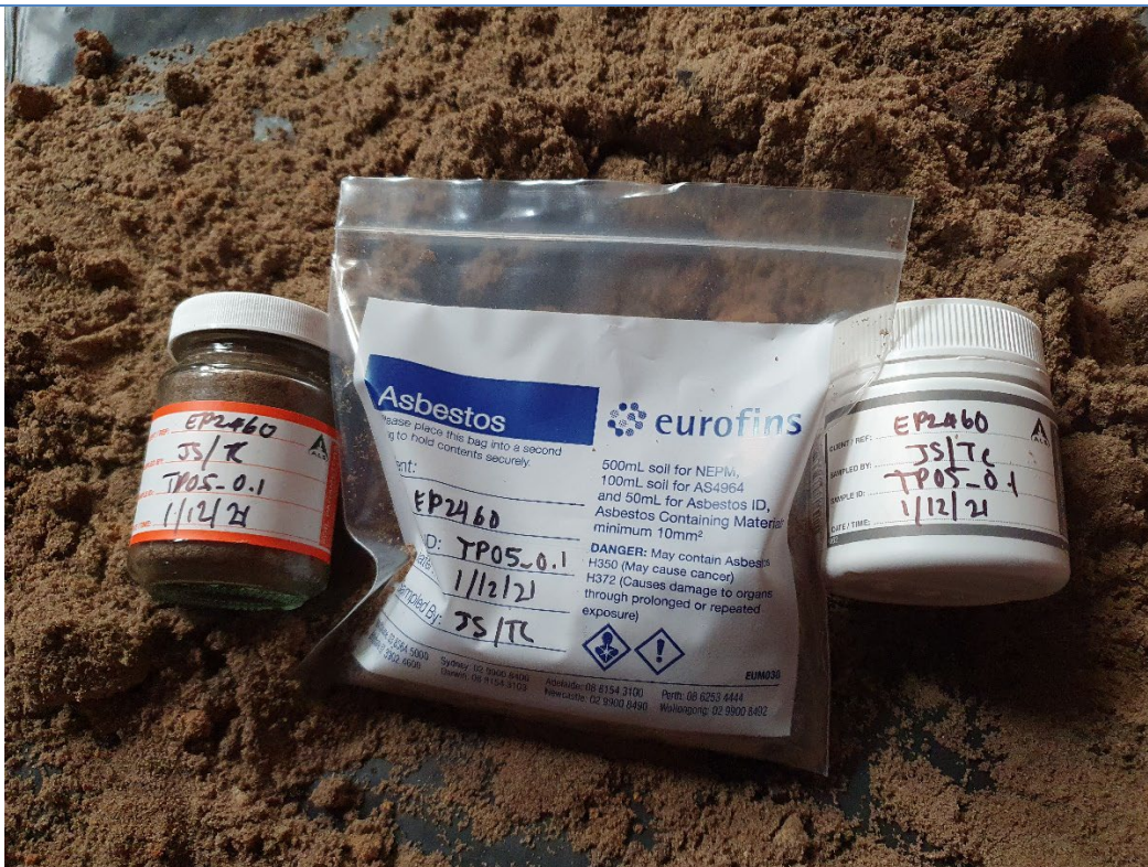
Plate 6 – Representative image of Soil material observed during SCA (EP Risk 2021): Gravelly sand, medium grained, angular to sub-angular gravels, light brown, slightly moist and loose.
