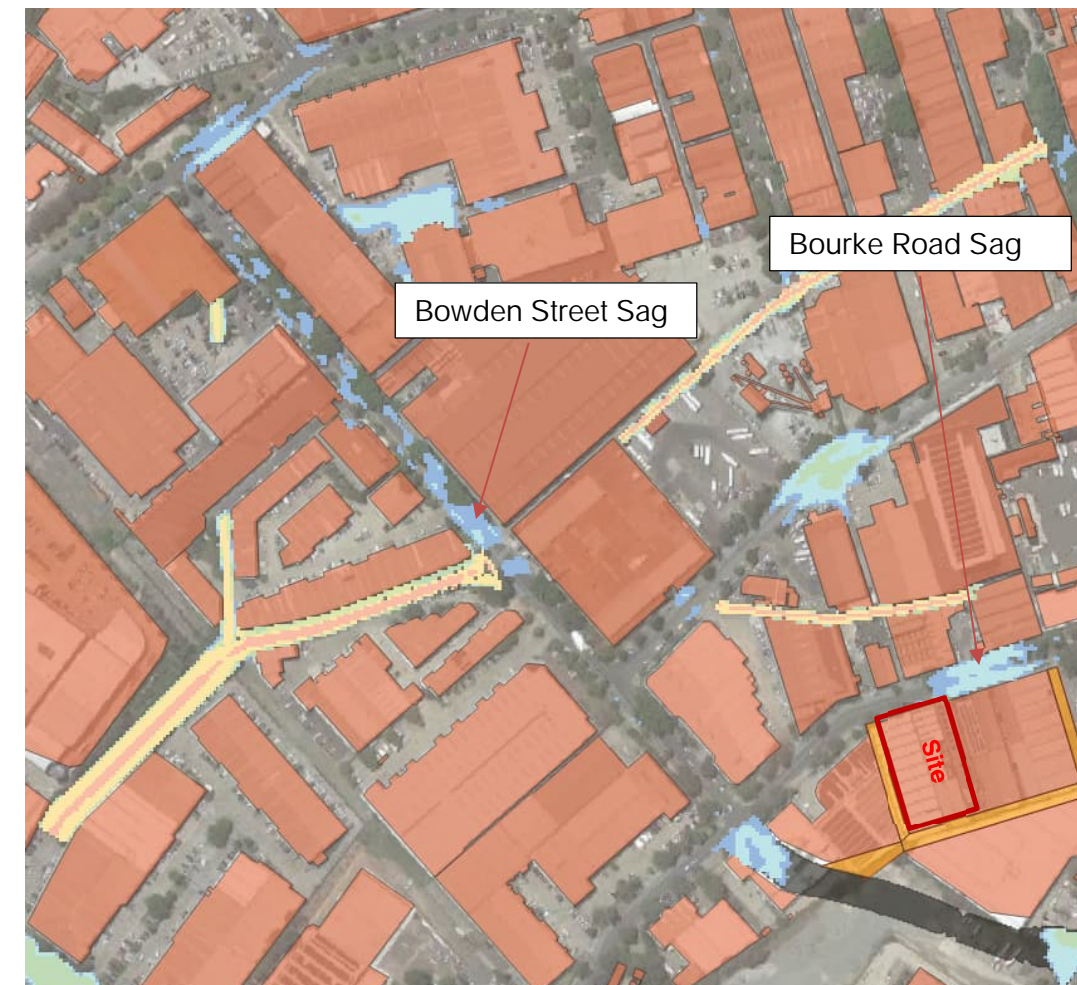
Figure 9 5% AEP flood hazard plot showing Bowden Street trafficable
