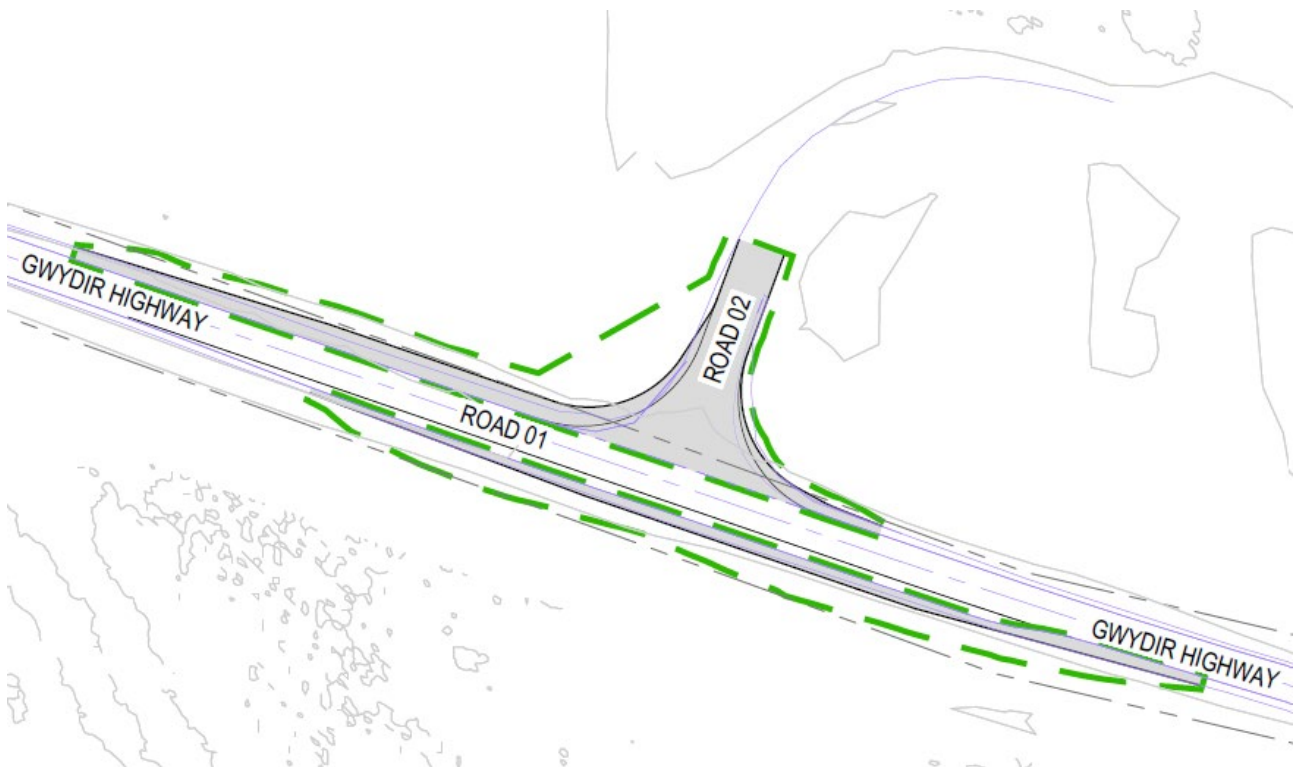
Figure 8.2 - Preliminary design of proposed turn treatment upgrade at the Wathagar Cotton Gin entry
