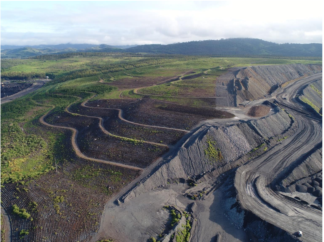
Figure 34: Newly completed rehabilitation at Mt Owen North Pit incorporating natural landform design. Note older rehabilitation areas in the background
