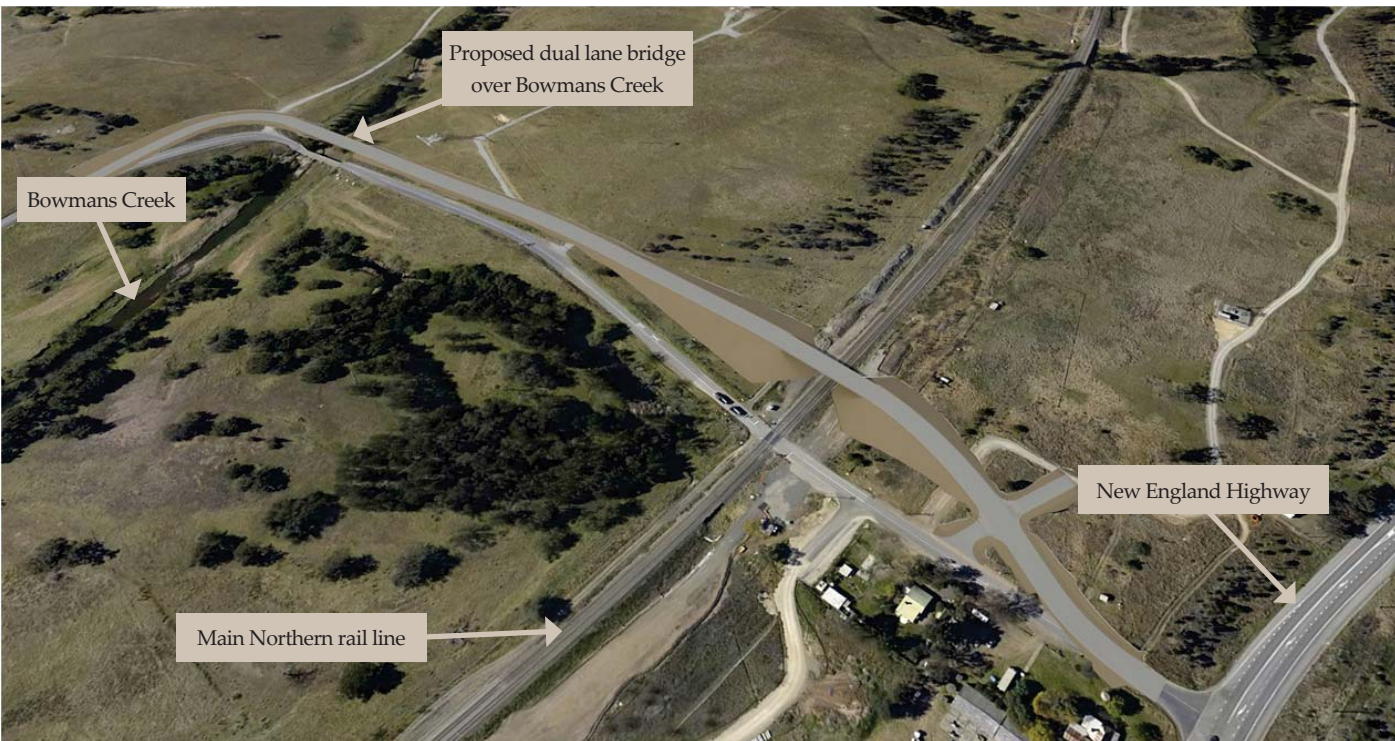
Proposed Hebden Road upgrade works.
