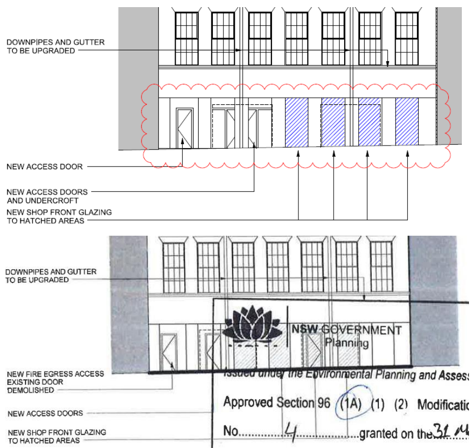
Figure 3 Proposed Wynyard Lane elevation (modifications bubbled red) on top, and the approved elevation on bottom (Mod 4)
