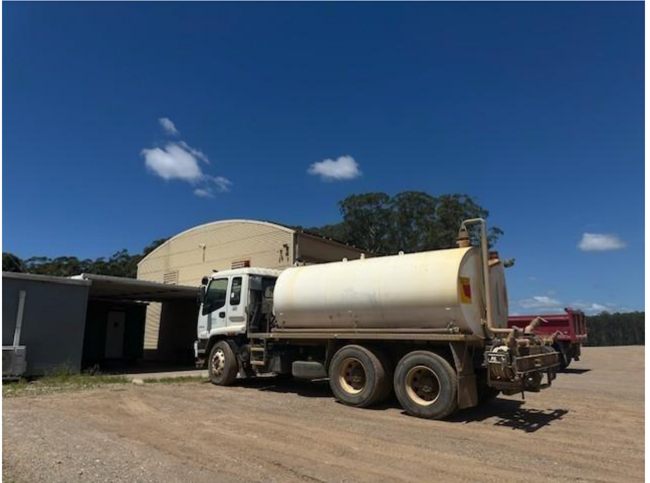
Water truck used for dust suppression.
