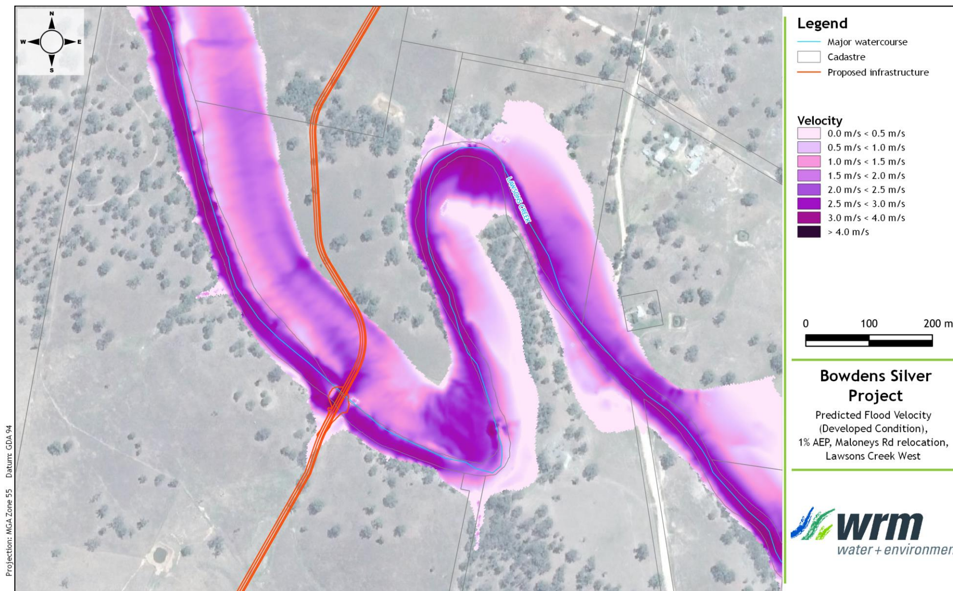
Figure 7.10 - 1% (1 in 100) AEP peak velocities along Lawsons Creek in the vicinity of the proposed Lawsons Creek Crossing - Lawsons Creek Crossing Scenario
