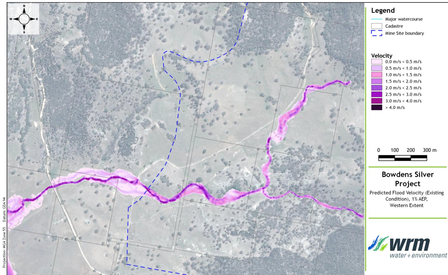
Figure 6.8 - 1% (1 in 100) AEP peak flood velocities - existing conditions - western extent
