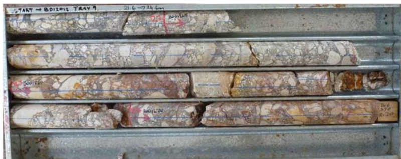
BD12012 Tray 9, 21.6m to 24.6m. Conglomerate, 07/03/2012 (21.3m to 22m, 0.6% S, 410ppm Mn and 35ppm Zn)
