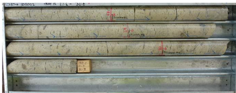
BD12002 Tray 12, 27.6m to 30.6m. Ignimbrite 07/03/2012 (28m to 29m, 0.4% S, 8290ppm Mn and 291ppm Zn)
