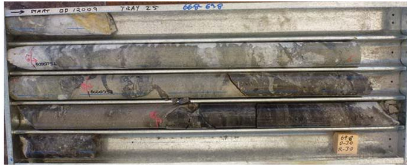
BD12009 Tray 25, 66.8m to 69.8m. Volcanic Breccia, 29/02/2012 (67m to 68m, 1.0% S, 1050ppm Mn and 3030ppm Zn)
