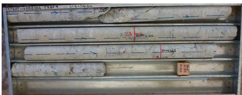
BD12009 Tray 9, 21.6m to 24.6m. Ignimbrite 07/03/2012 (22m to 23m, 1.7% S, 2460ppm Mn and 4600ppm Zn)
