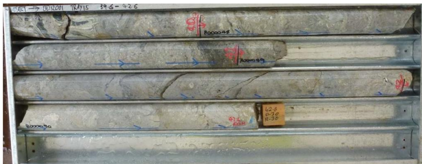
BD12001 Tray 15, 39.6m to 42.6m. Volcanic Breccia, 02/02/2012 (40m to 41m, 0.5% S, 543ppm Mn and 1995ppm Zn)
