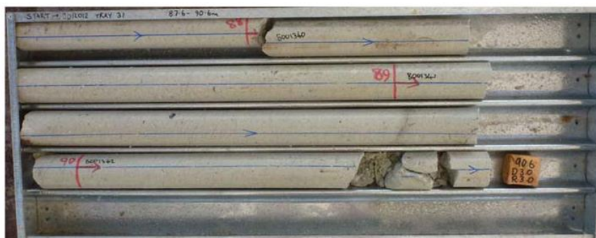
BD12012 Tray 31, 87.6m to 90.6m. Ignimbrite. 07/03/2012 (87m to 88m 0.0% S, 4680ppm Mn and 133ppm Zn)
