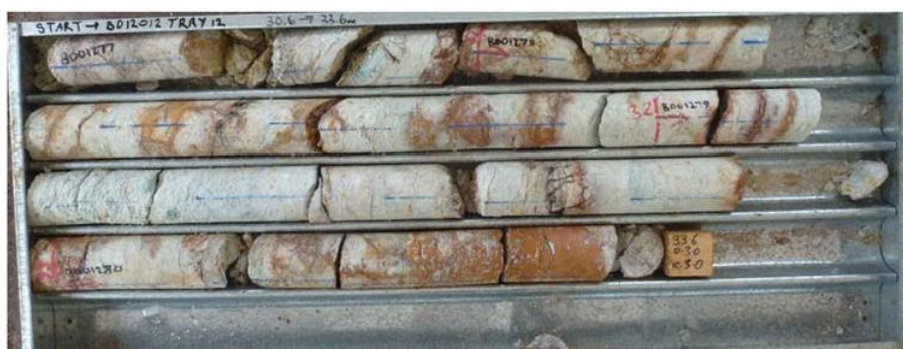
BD12012 Tray 12, 30.6m to 33.6m, Crystal Tuff, 07/03/2012 (33m to 34m, 0.1% S, 1015ppm Mn and 115ppm Zn)
