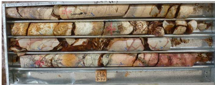
BD12011 Tray 12, 30.7m to 33.7m. Crystal Tuff 02/06/2012 (33m to 34m, 0.1% S, 125ppm Mn and 40ppm Zn)
