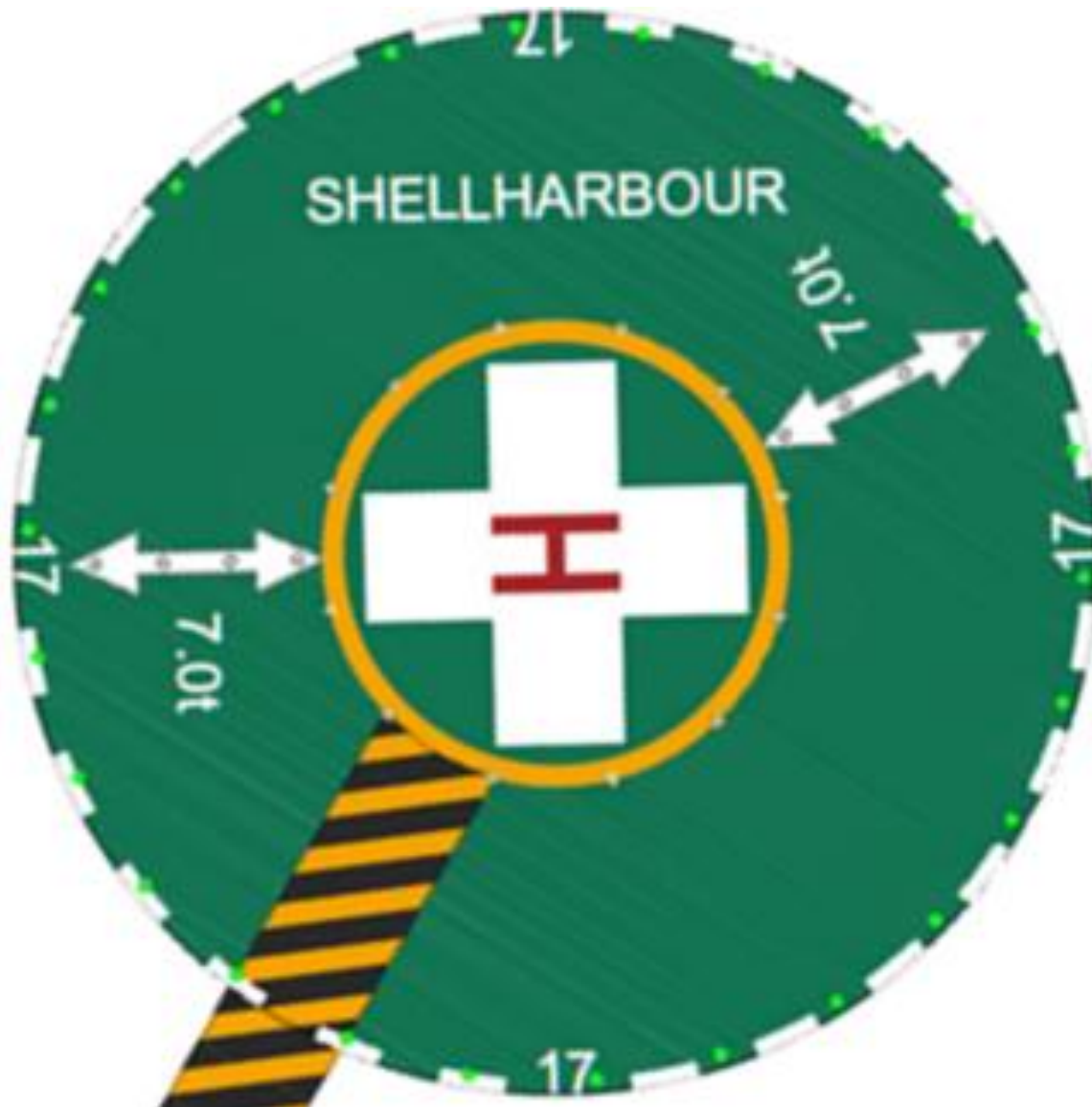
Figure 11: NSH HLS Design and Markings
