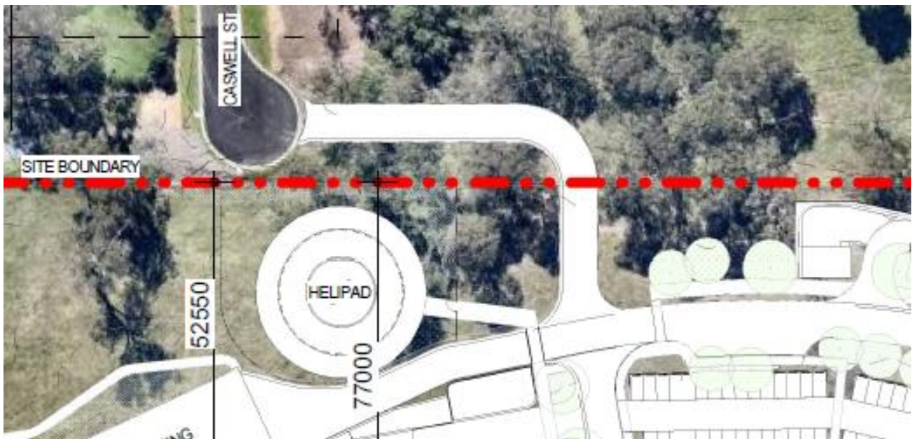
Figure 4.4: Secondary Controlled Access Location and Arrangement
