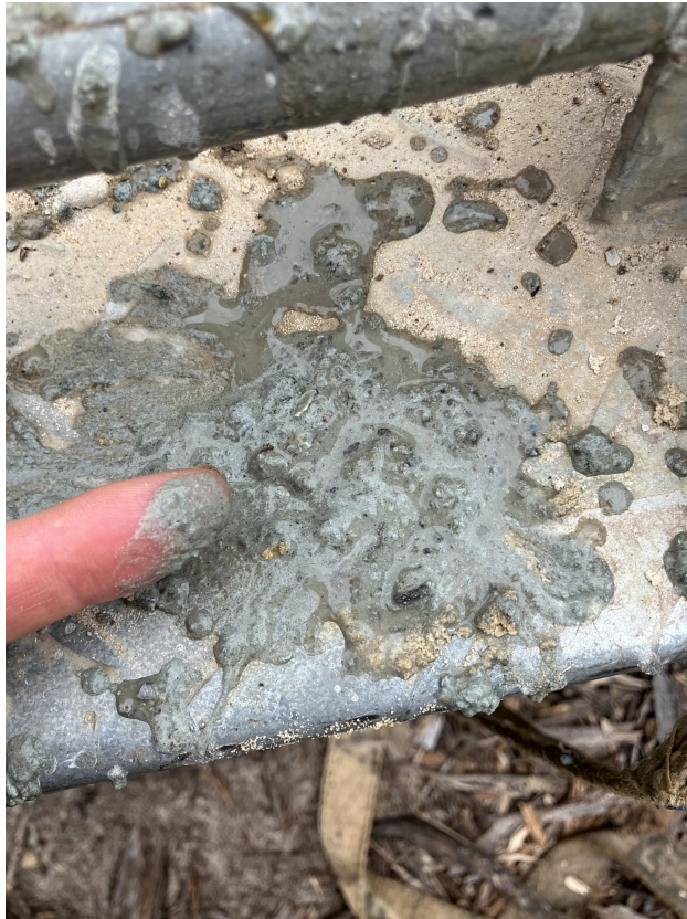
Sample 3 (Clayey SAND) - 17.50mbgl to 23.00mbgl
