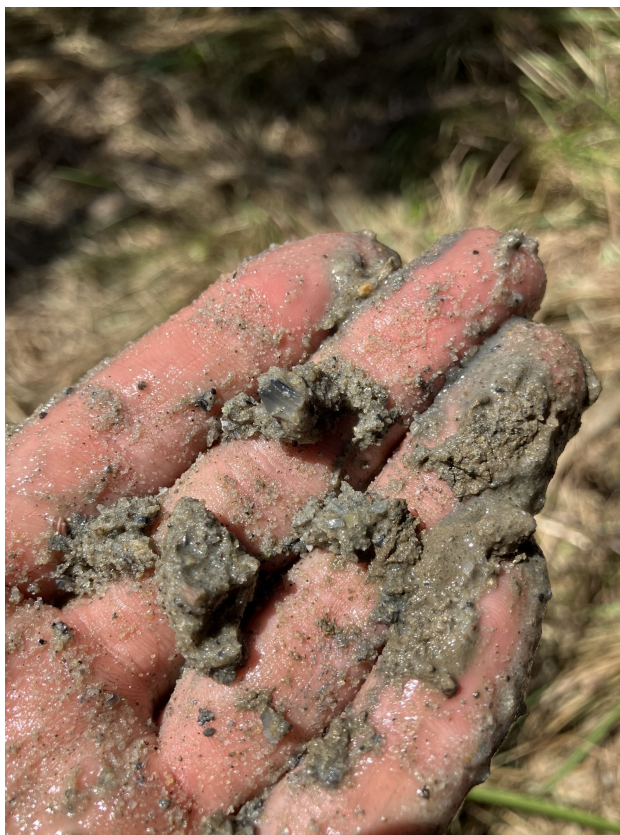
Sample 1 (clayey silty GRAVEL) - 6.50mbgl to 7.50mbgl
