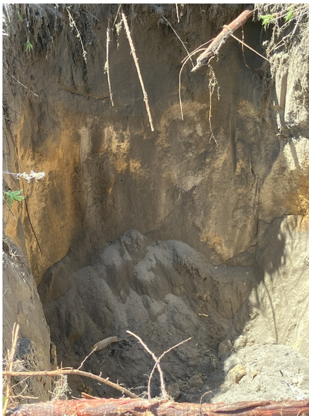
Test Pit - 0.00mbgl to 1.20mbgl
