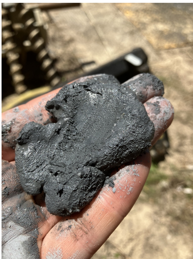
Sample 4 (silty CLAY, with sand) - 27.00mbgl to 30.00mbgl
