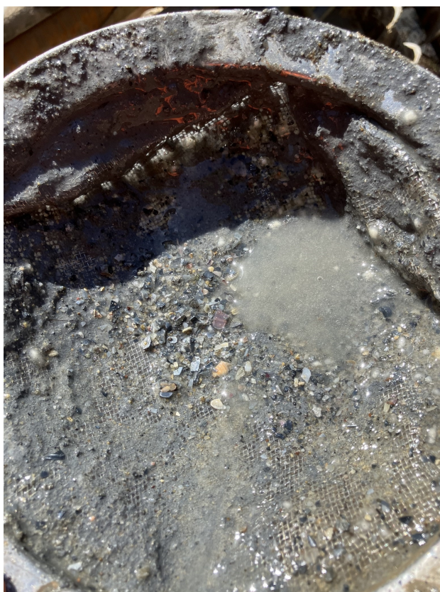
Sample 2 (clayey silty GRAVEL) - 7.00mbgl to 9.50mbgl
