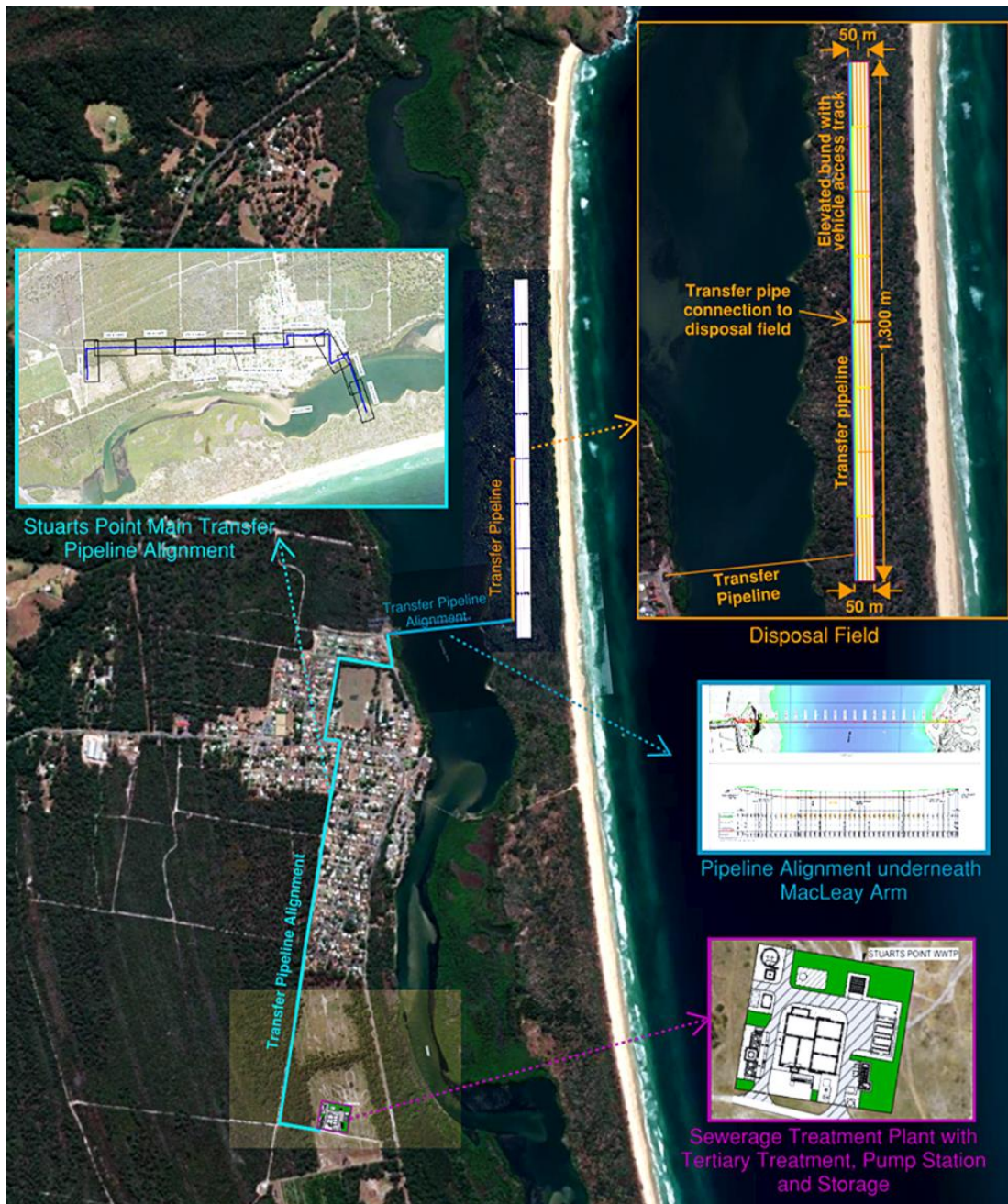
Figure 4 SPWWTP Treated Effluent Management System Overview
