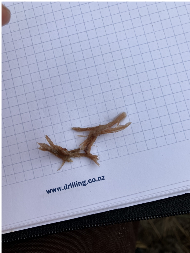
Sample 2 (fibrous tree root) - 7.00mbgl to 7.30mbgl
