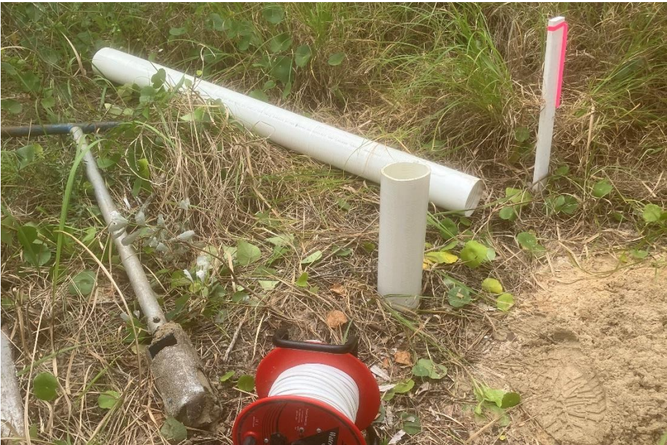
Figure 2-1. Photo of hand auger and perforated PVC pipe ready for infiltration testing.
