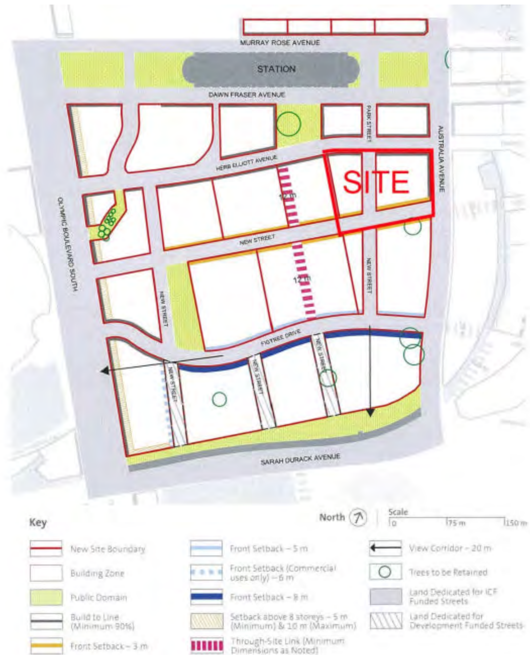
Figure 13. Central Precinct building zones and setbacks plan, Master Plan 2030 The subject site is shown with a red outline.
