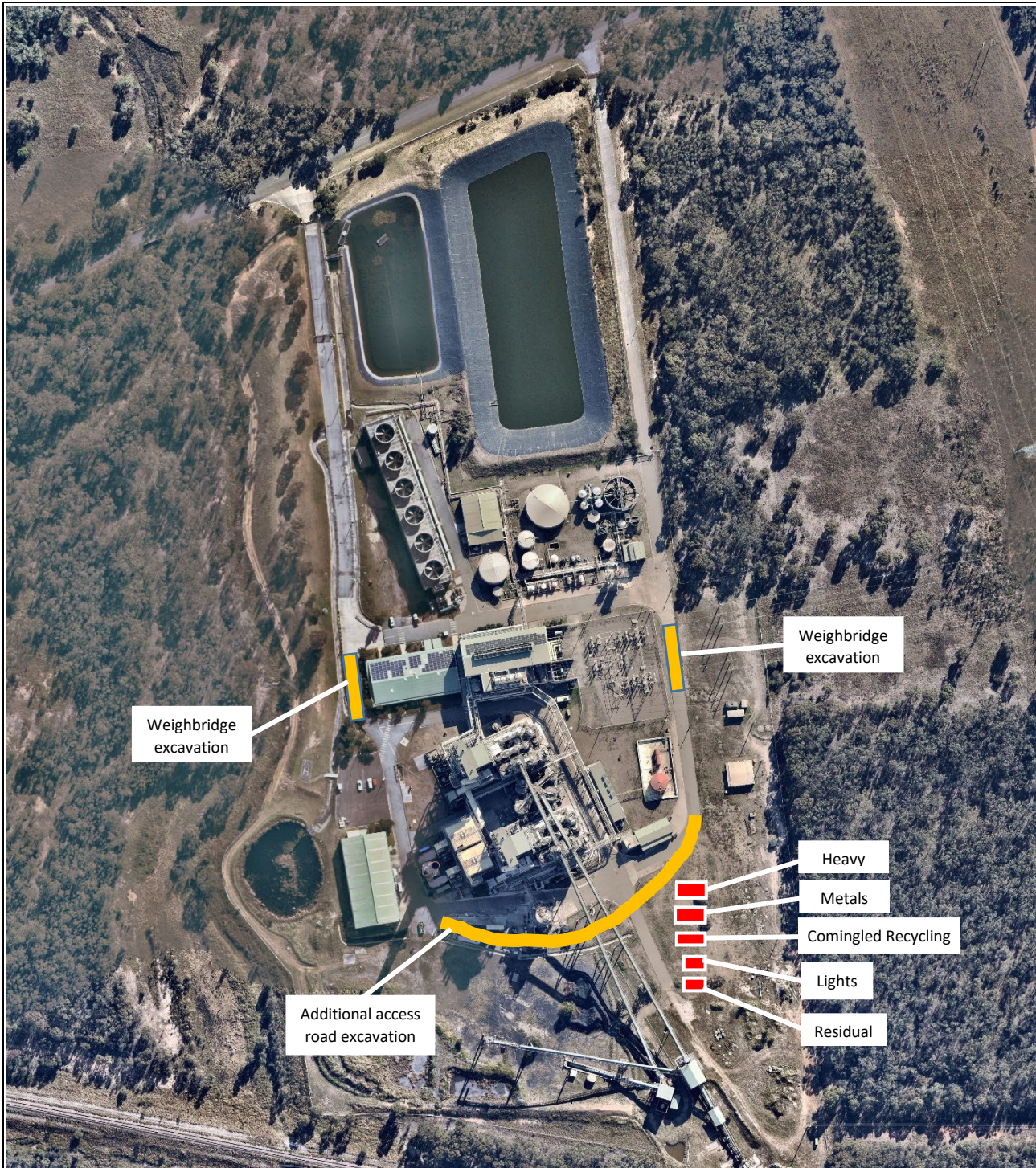
Figure 8.1. Areas to be excavated during construction in yellow boxes. Placement of waste storage and recycling bins during the construction phase in red boxes.
