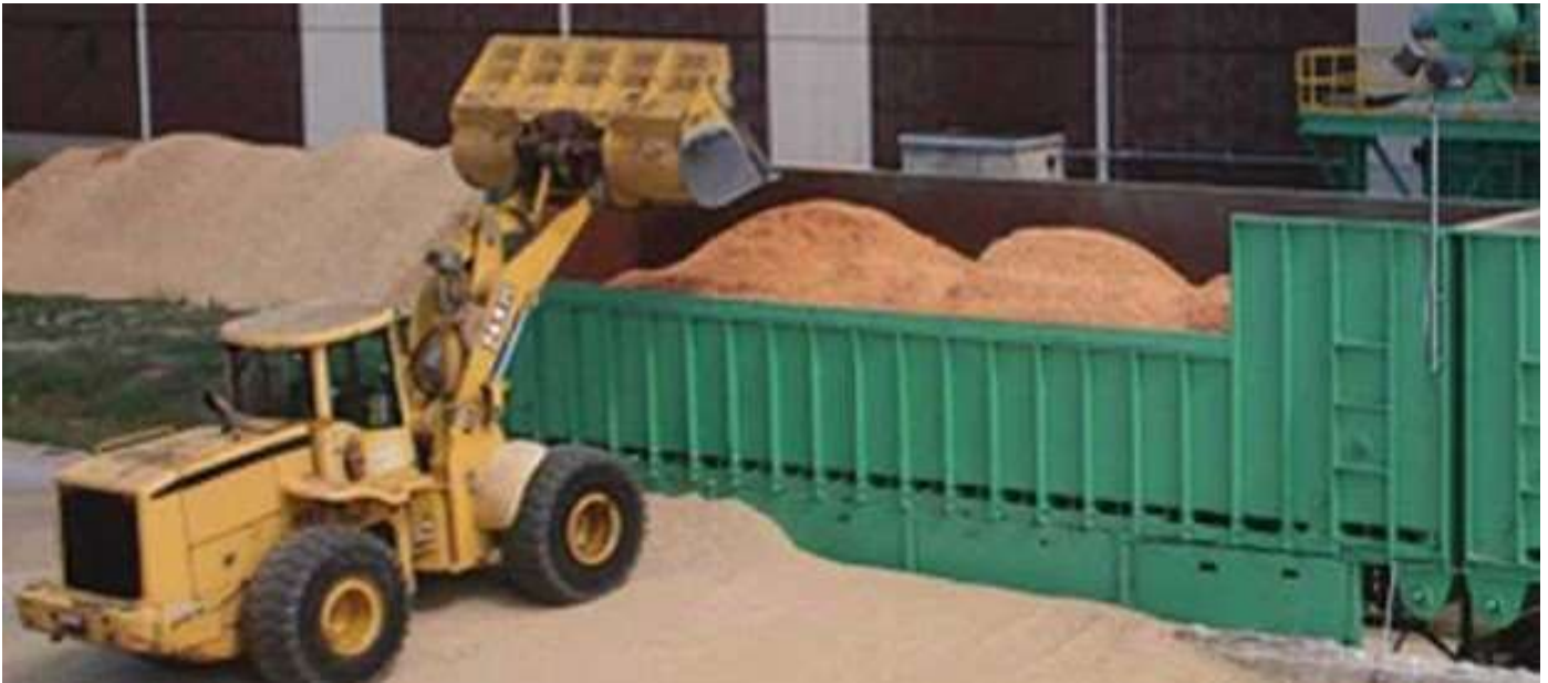
Figure 3.6. Moving floor bulk unloader bin.
