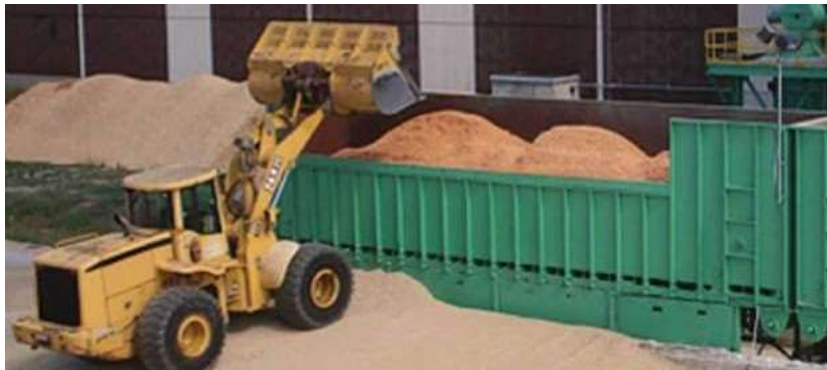
Figure 12 - Moving Floor Bulk Unloader Bin
