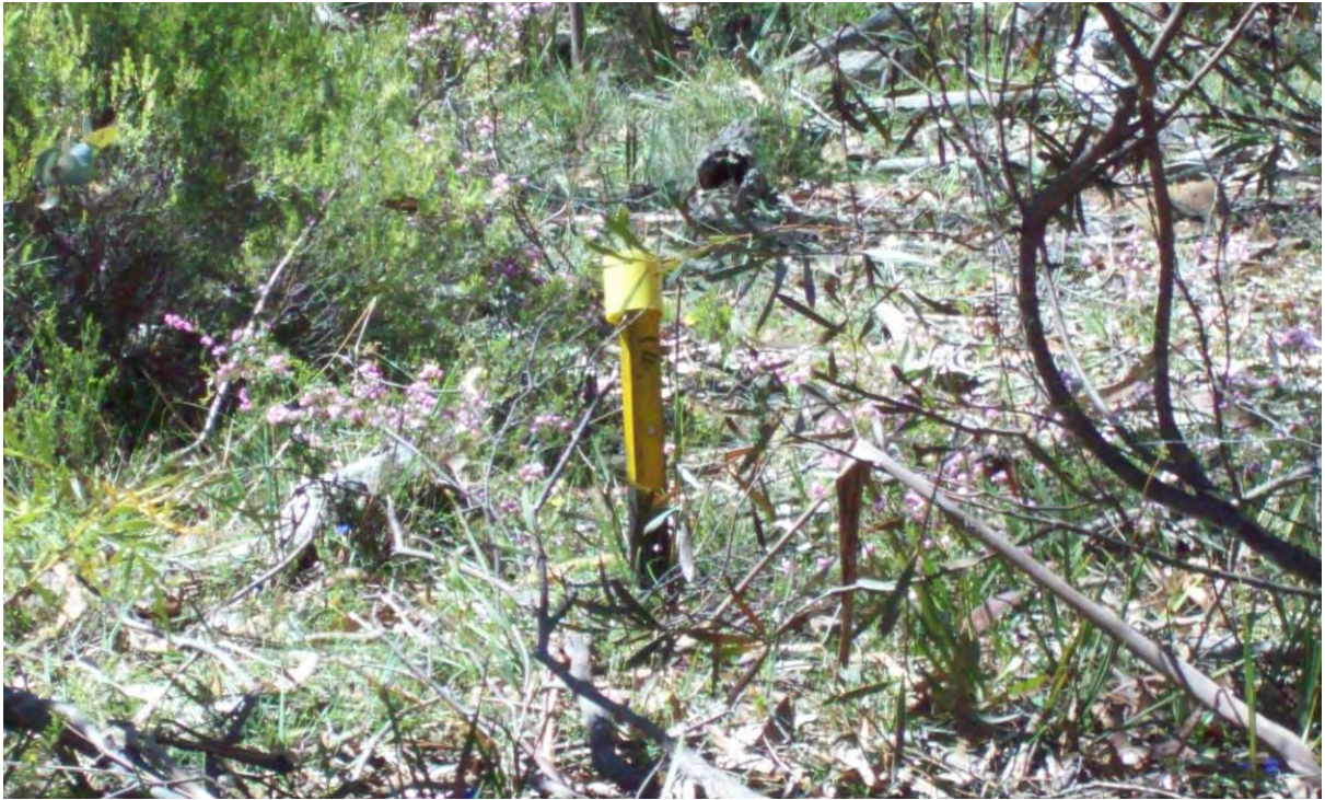
Plate 7: Subsidence Monitoring Peg
